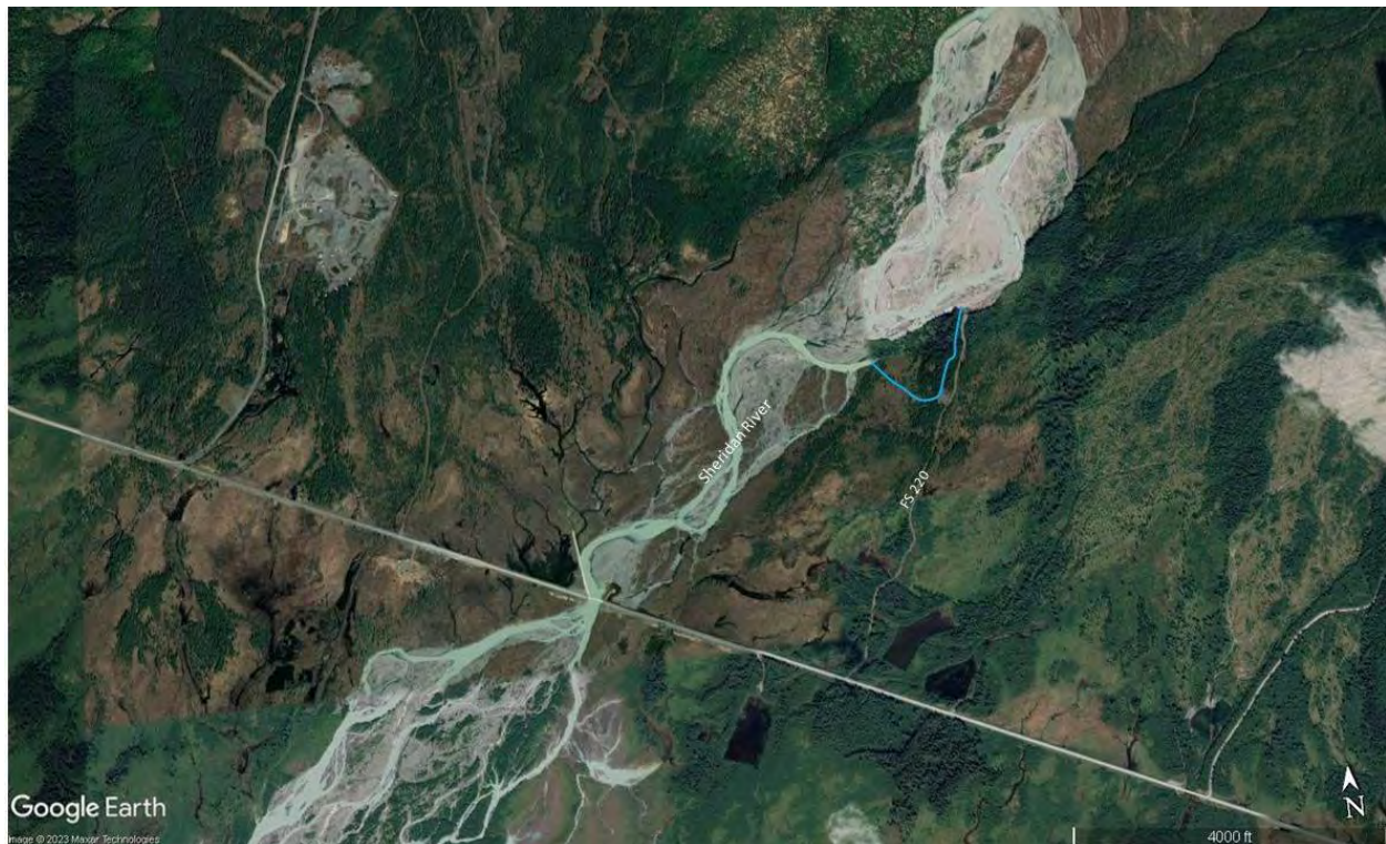
Image 1: An aerial image illustrating channel constriction. Blue line is the new path carved by the river in the last 2 years.
