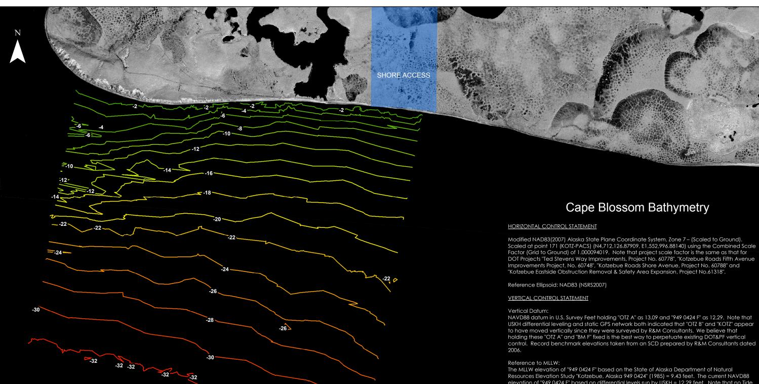
Resources Elevation Study "Kotzebue, Alaska 949 0424" (1985) = 9.43 feet. The current NAVD88 elevation of "949 0424 F" based on differential levels run by USKH = 12.29 feet. Note that no Tide study has been performed at Cape Blossom.
