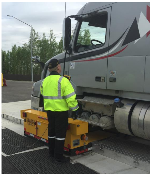
Above: A Commercial Vehicle Enforcement Officer testing the brakes on a CMV using the Performance Based Brake Tester (PBBT).
