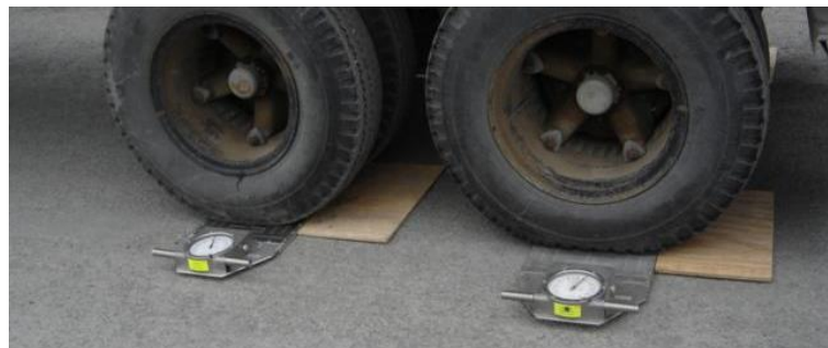
Haenni scales weighing a double axle.
