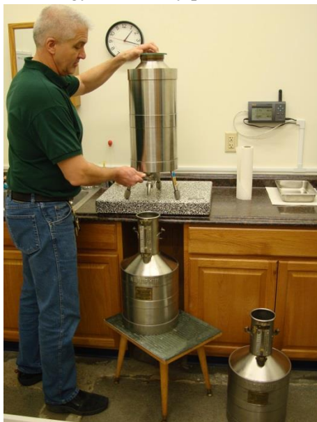
Above: State Metrologist Roger Holland calibrating a five gallon neck type prover using the NIST traceable slicker.
