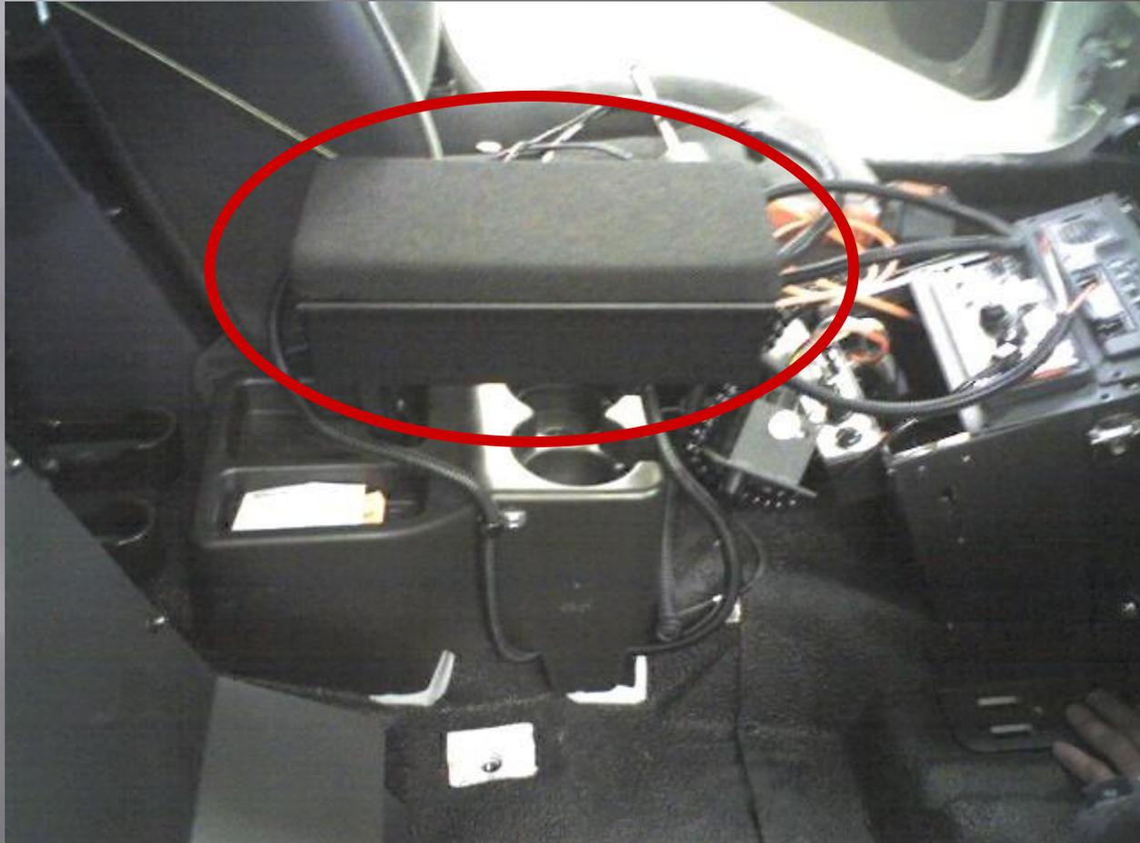
**The Printer in most newer Impalas will be mounted in this location and can be swiveled to the side and tilted back for access to the OE Console**
