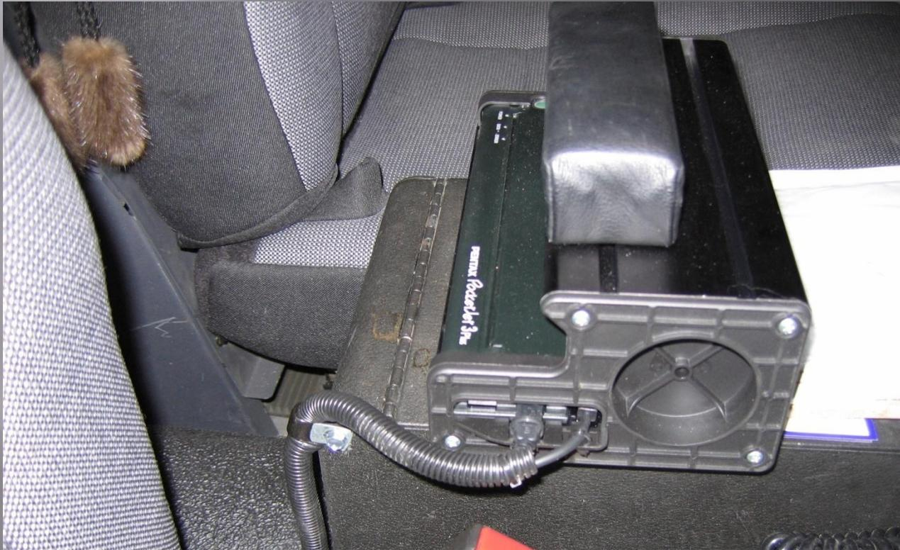
**The Printer will be mounted in this location for most typical installations. We must be able to free up the area on the rear of the console to facilitate this type of mount. Some installations will require the removal of cup holders or storage pockets on the console.**
