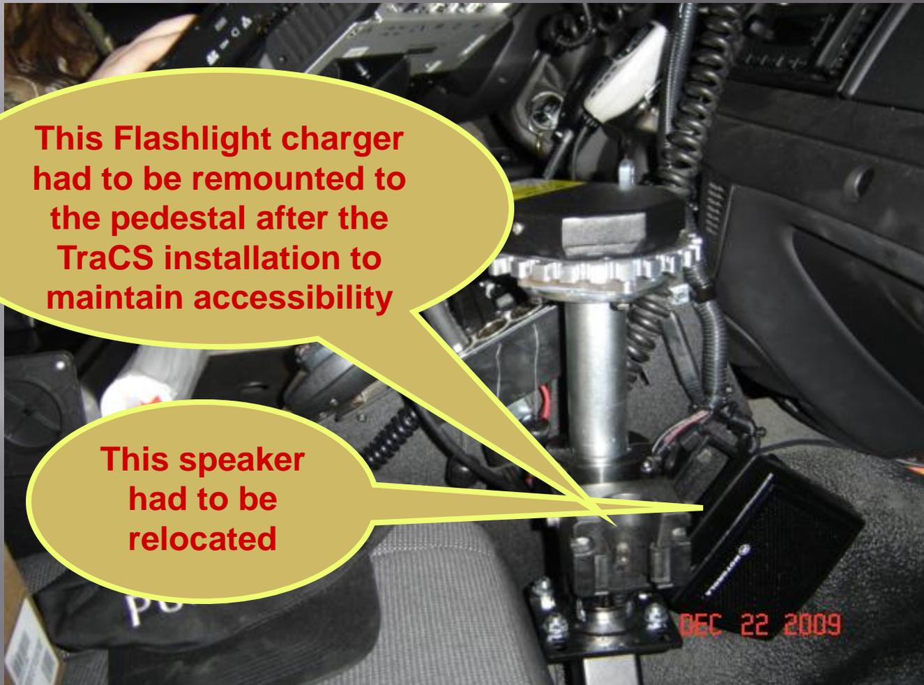
**This Flashlight charger had to be remounted to the pedestal after the TraCS installation to maintain accessibility**
