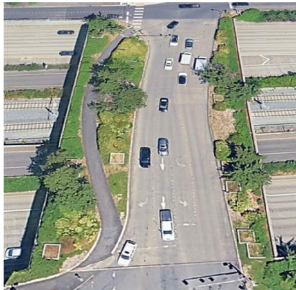
This image depicts the concept proposed for crossings of Karluk and Medfra Streets. The extra-wide bridges would allow for a separated trail and landscaping and shield the surface users from the traffic below.
