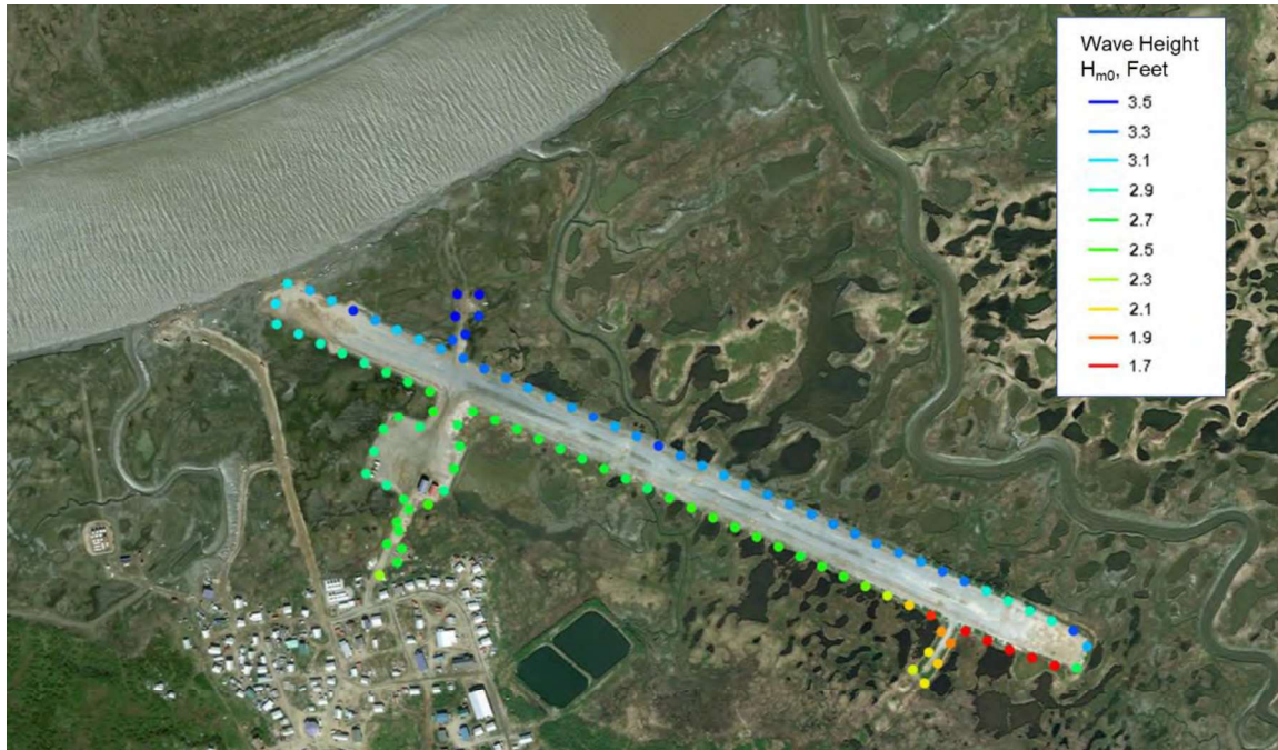
Figure 14: Spectral Significant Wave Height Results at Scammon Bay Airport
