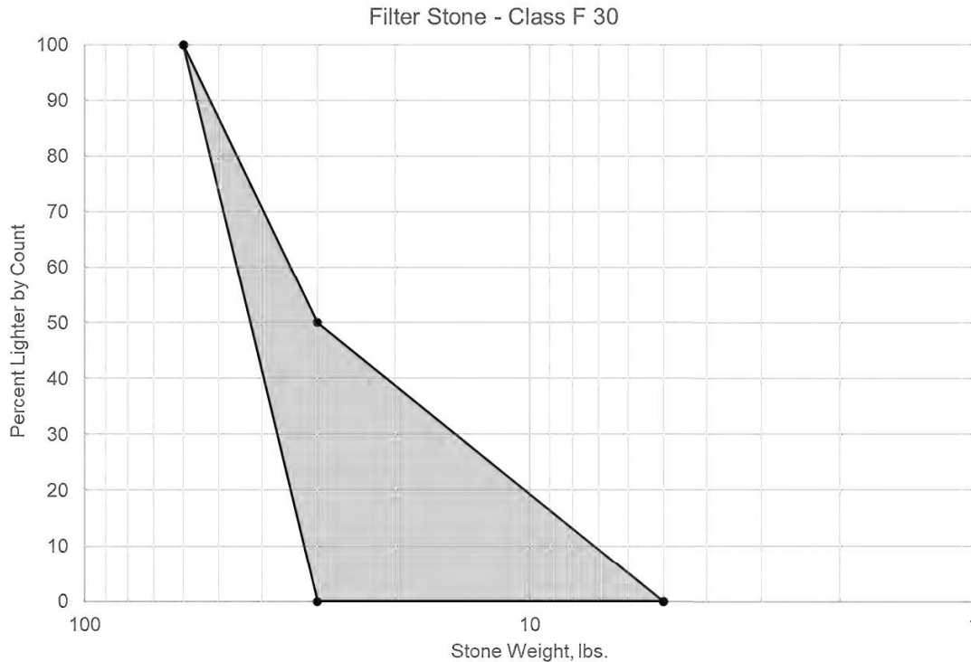
Figure 19: Recommended Filter Stone Gradation (F-30)
