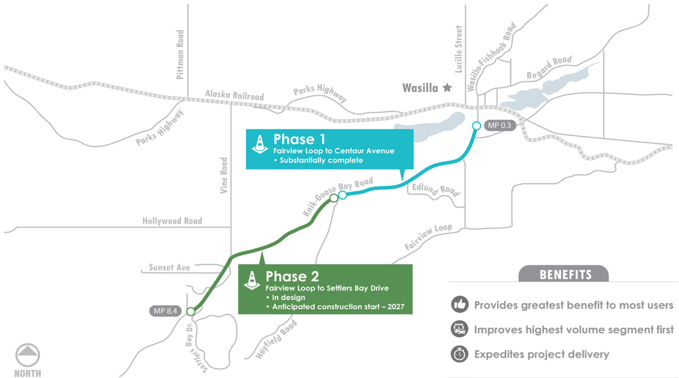
Figure 2: Construction Phasing Plan
