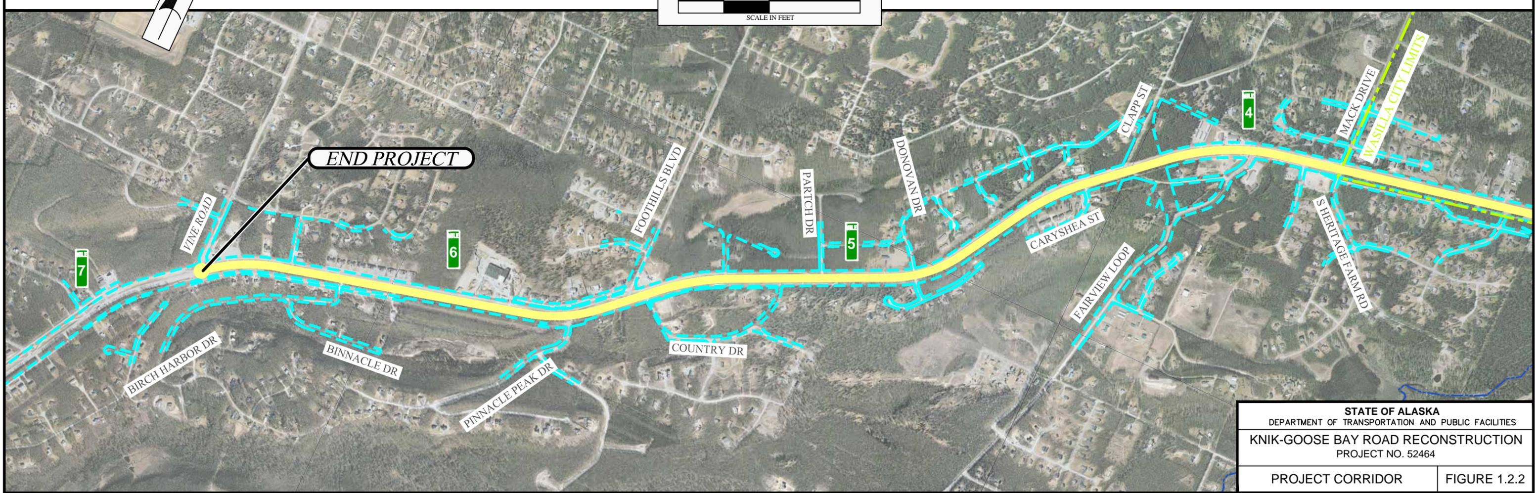
The intersections of PWH, Fern Street, Fairview Loop Road, and Vine Road are signalized and have illumination. All remaining street approaches are stop-sign controlled. All intersections are illuminated along the corridor. The following eight intersections have auxiliary turn lanes:
