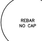
(813) Found 1/2" rebar, projecting 0.3' above the ground, no cap. Good
