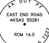
(24) Set 2 1/2"x30" alum. post, 30" in the ground, with  $3 \frac{1}{4}$ " alum. cap marked as shown, with a clear magnet at base. Carsonite post S50°E, 1.0 ft.
