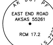
Set 2 1/2"x30" alum. post, 29" in the ground, with 3 1/4" alum. cap marked as shown, with a clear magnet at base. Carsonite post N30°W, 1.0 ft.
