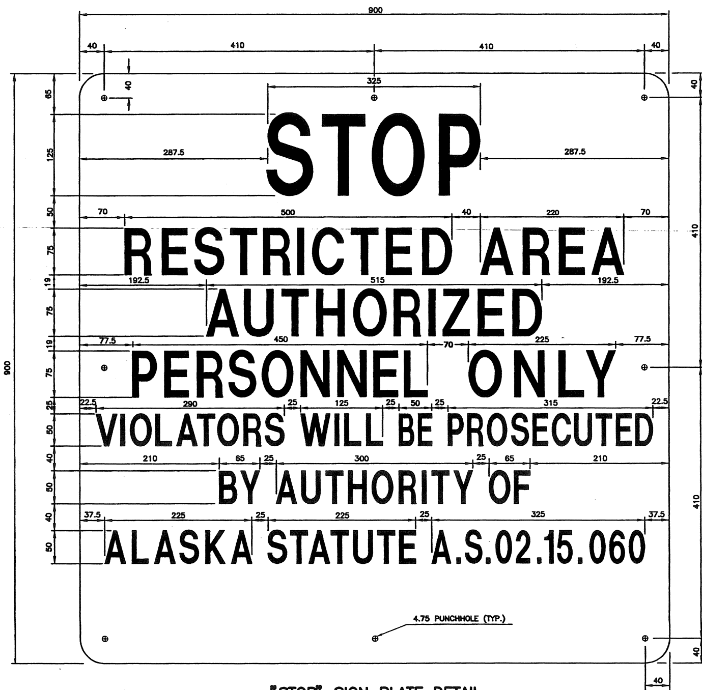
"STOP" SIGN PLATE DETAIL NO SCALE
