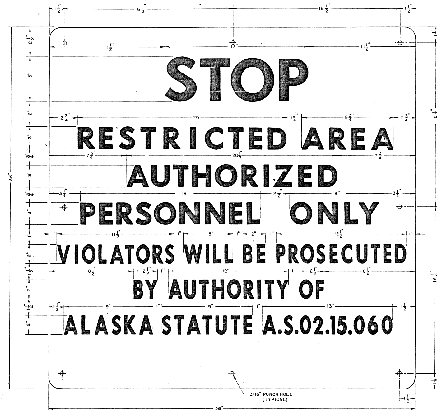
"STOP" SIGN PLATE DETAIL
