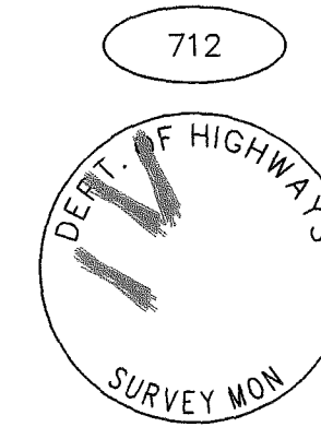
Fnd 2-1/2" Brass Cap in Monument Case 0.5' Below Grade Good Condition
