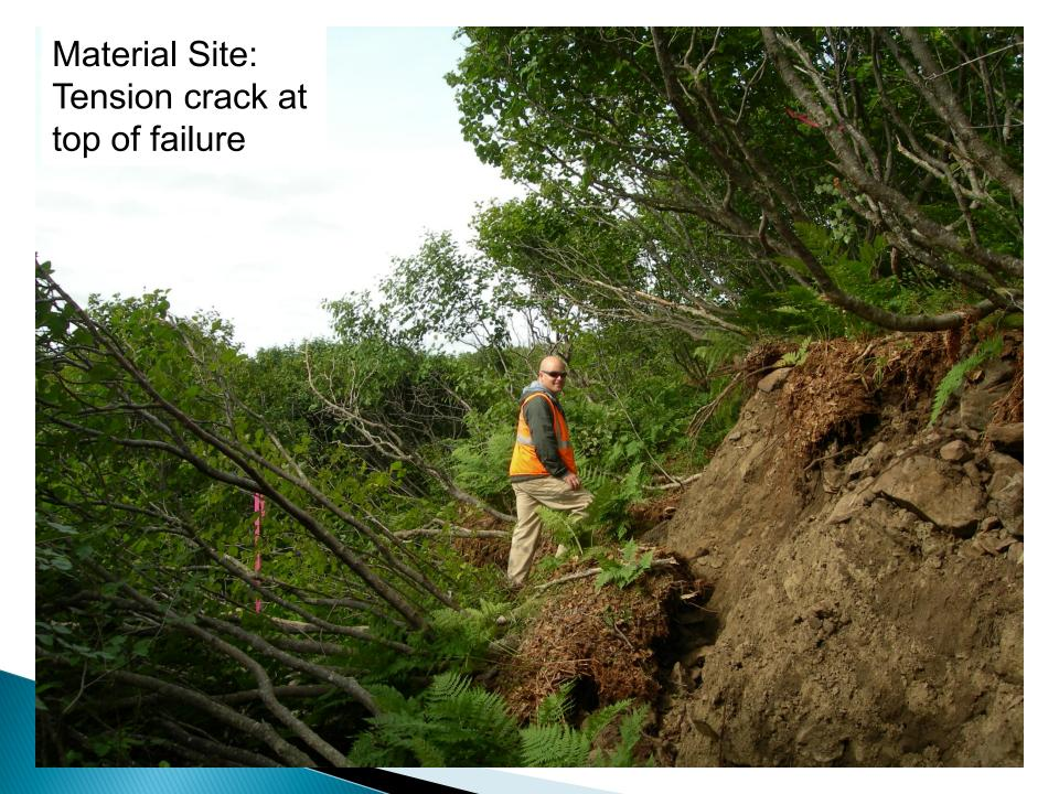
Material Site: The contractor went up to the Talus Area and excavated boulders for processing. Either because of the slope failure (they unloaded the slope), less drainage issues, or to get better quality rock.
