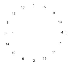
After torquing the top nuts, use a hydraulic wrench to rotate top nuts an additional one third (120°) turn, while preventing the leveling nuts from turning. Use the crisscross pattern shown above.
