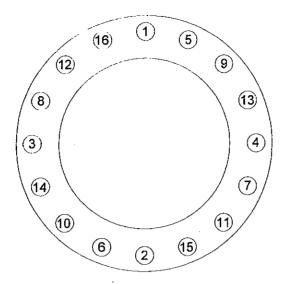
After torquing the top nuts, use a hydraulic wrench to rotate top nuts an additional one sixth  $(60^{\circ})$  turn, while preventing the leveling nuts from turning. Use the crisscross pattern shown above.
