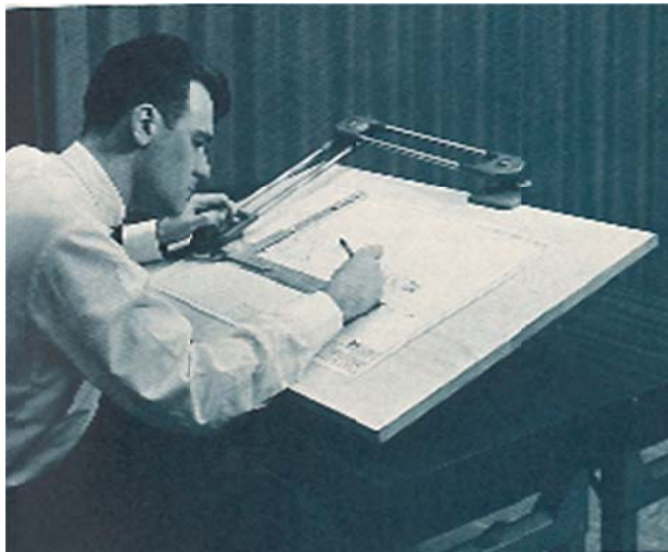
Figure 11. Drafting Machine. Source: Technical Drawing, Seventh Edition, 1980
