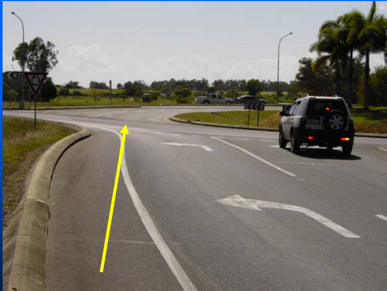
Circulatory road is narrowed to one lane to guide drivers to select correct lane
