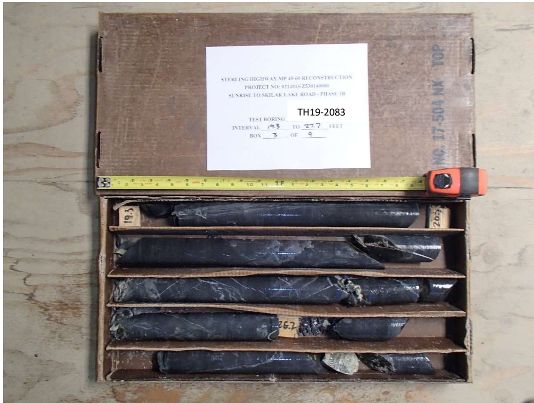
Test Boring TH19-2083, Interval 19.3 to 27.7 ft, Box 3 of 9
