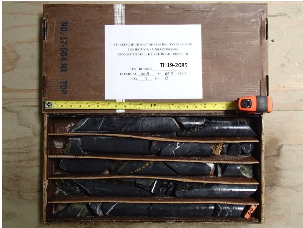
Test Boring TH19-2085, Interval 56.8 to 65.0 ft, Box 7 of 8
