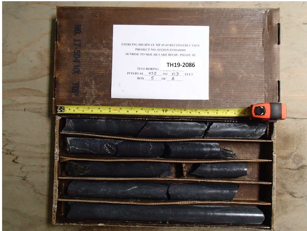
Test Boring TH19-2086, Interval 43.0 to 51.3 ft, Box 5 of 6
