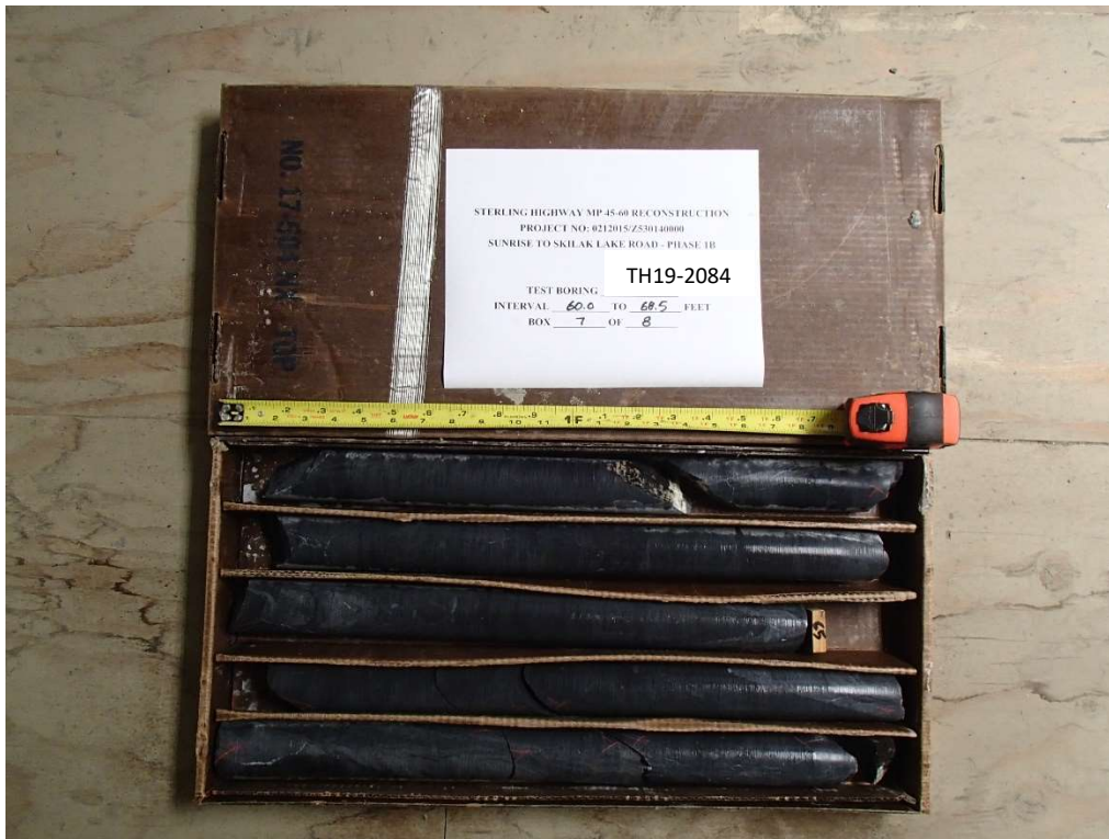
Test Boring TH19-2084, Interval 60.0 to 68.5 ft, Box 7 of 8
