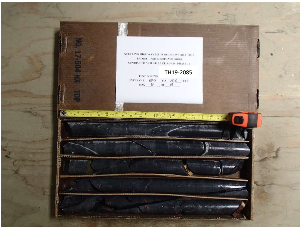
Test Boring TH19-2085, Interval 65.0 to 75.0 ft, Box 8 of 8
