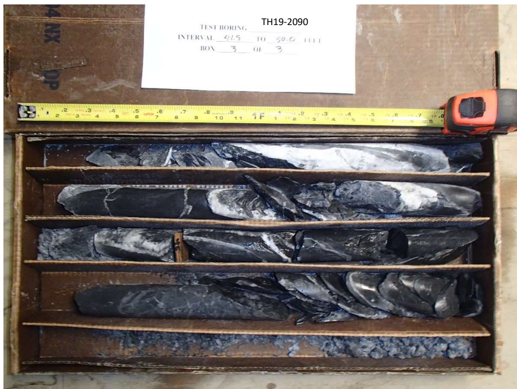
Test Boring TH19-2090, Interval 41.5 to 50.0 ft, Box 3 of 3
