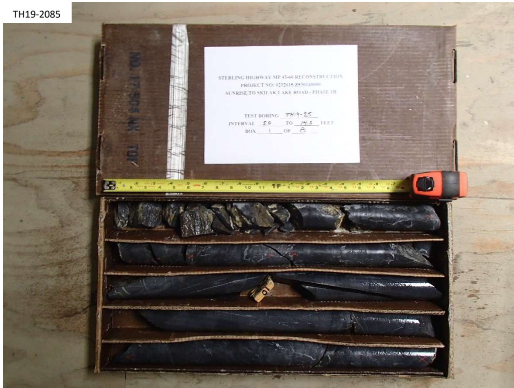
Test Boring TH19-2085, Interval 5.0 to 14.0 ft, Box 1 of 8
