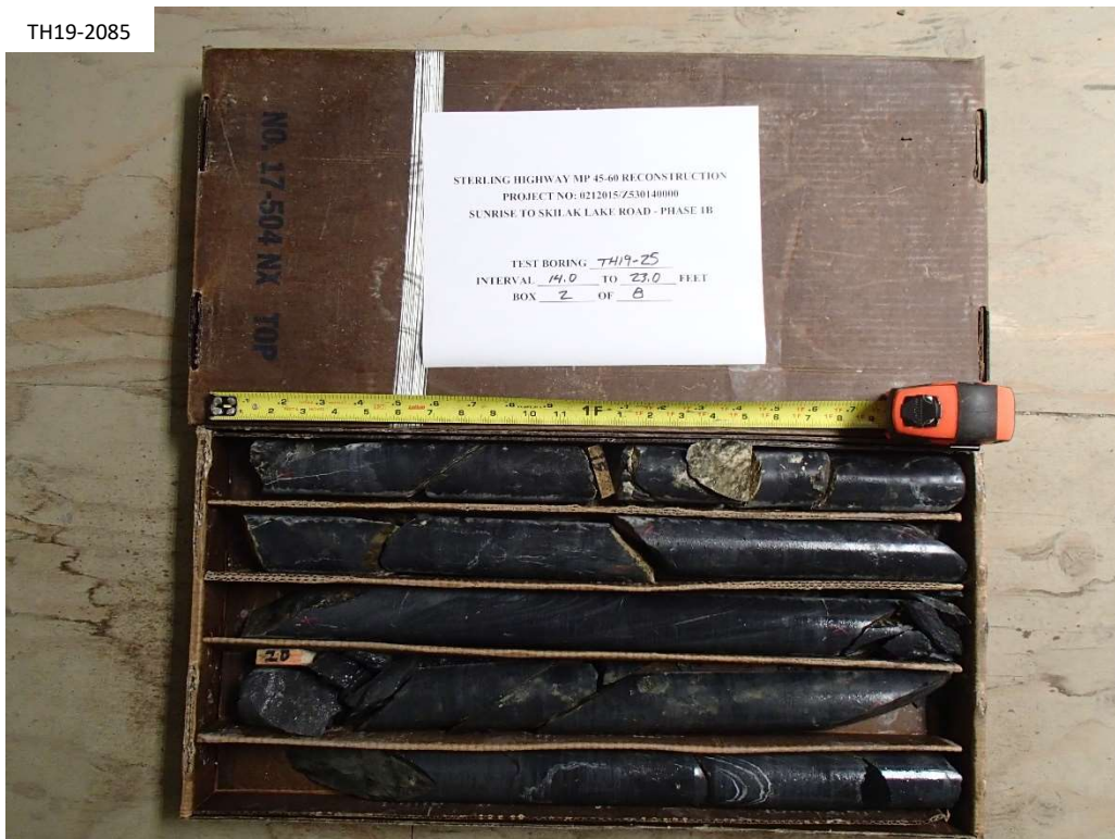
Test Boring TH19-2085, Interval 14.0 to 23.0 ft, Box 2 of 8
