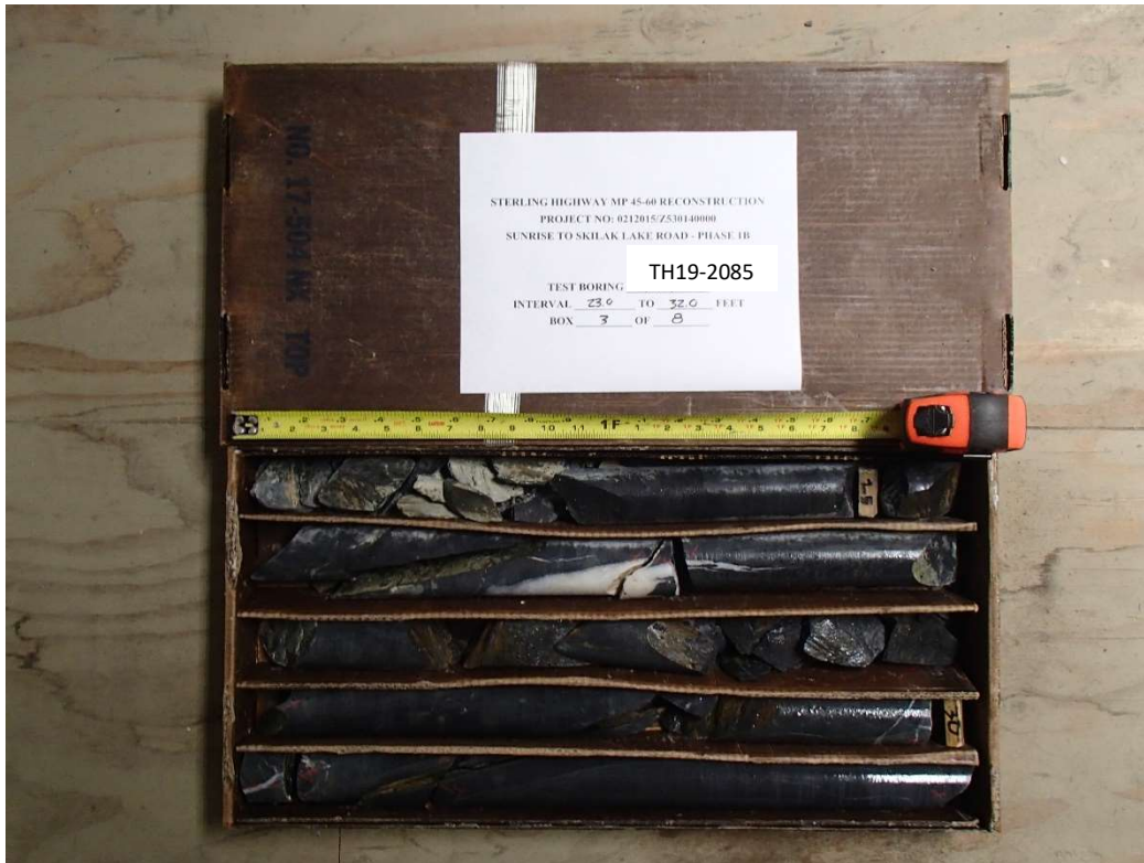
Test Boring TH19-2085, Interval 23.0 to 32.0 ft, Box 3 of 8
