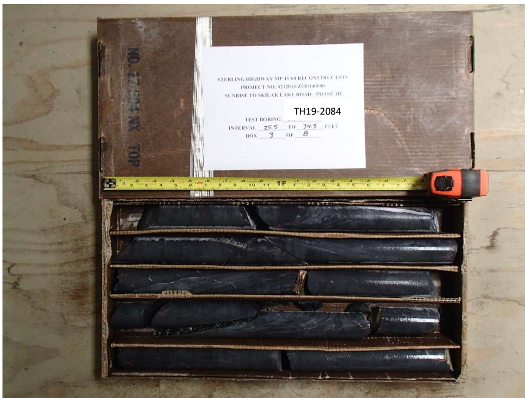
Test Boring TH19-2084, Interval 25.5 to 34.5 ft, Box 3 of 8
