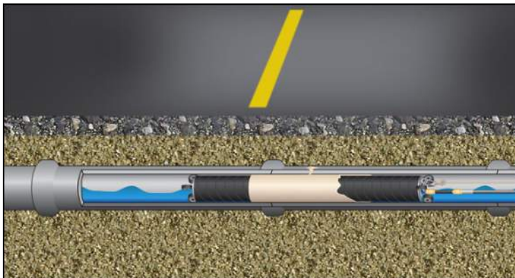
Trenchless point repair (courtesy of Pipe Patch).
