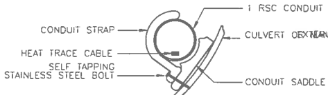
4 CONDUIT SUPPORT DETAIL SCALE: NONE MANHOLE SUPPORT SIMILAR
