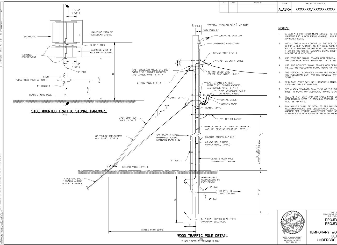
ATTACH A 4 INCH RIGID METAL CONDUIT TO THE WOOD POLE, USING UNISTRUT P9014 WITH P4101 CHANNEL, AND P1121 PIPE CLAMPS, OR APPROVED EQUAL.
