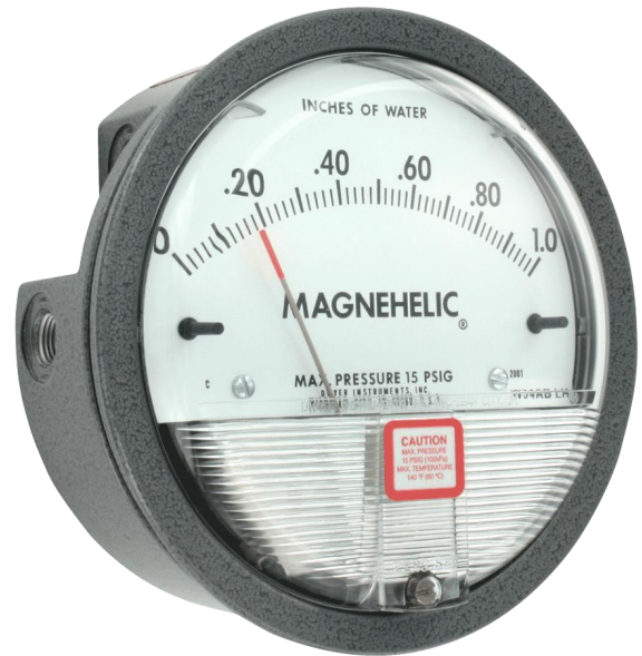
Magnehelic® Differential Pressure Gauge (0 - 1" model shown)
