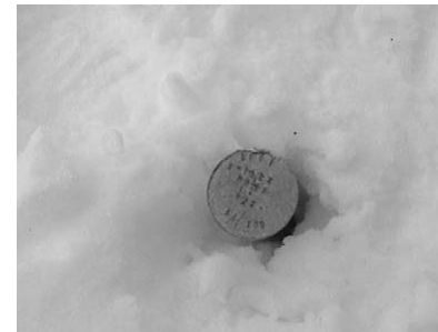
Photo 1 – Runway Station Monument, Rebar and Cap
