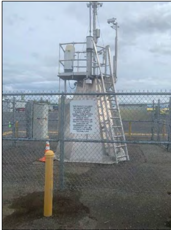
Figure 15: Automated Weather Observation System
