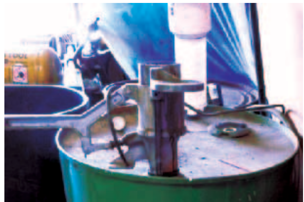
Use an aerosol can puncturing device, for example this one mounted over a hazardous waste drum, to safely drain the contents of your aerosol cans
