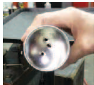
Use an aerosol can puncturing device, for example this one mounted over a hazardous waste drum, to safely drain the contents of your aerosol cans
