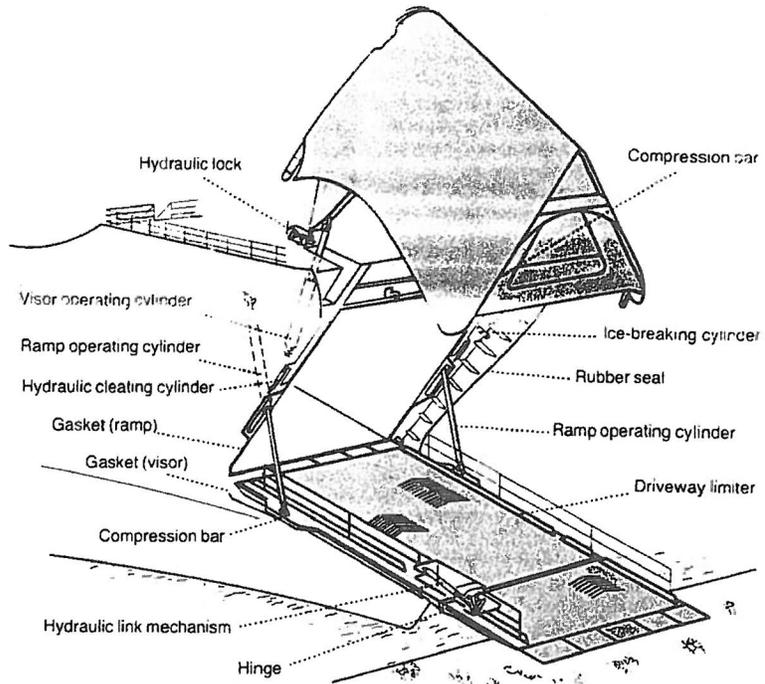
Visor design usually results from a collaboration between MacGregor-Navire and the shipyard—and its supply is also a divided responsibility, with the yard supplying the structure itself and MacGregor-Navire being responsible for the actuating mechanism, i.e. the hydraulic and mechanical parts and components. This is a convenient arrangement since the visor is
