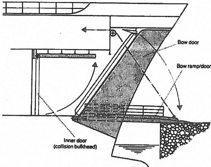
About one third of all ships on unrestricted service which have a roll-on, roll-off capability, incorporate access by the bow as well as by the stern. Most of these are car/passenger ferries which, for quick turnaround, need the 'drive through' facility thus made possible; but bow access is also invaluable on some other, less numerous, ship types such as train ferries, naval support ships (e.g. LST's, dock hold ships) and heavy lift vessels.
