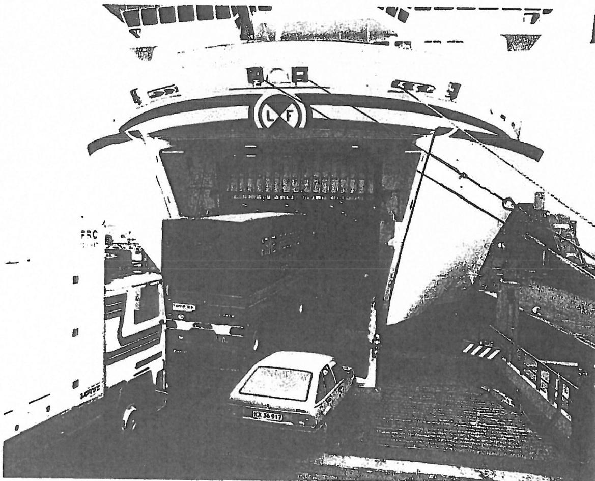
Usually, forward access ramps are constructed in two or three sections which fold into stowage well behind an outer closure. Here, careful design is necessary since the available stowage space – which may have to accommodate a two- or three-piece folded ramp – is often restricted.
