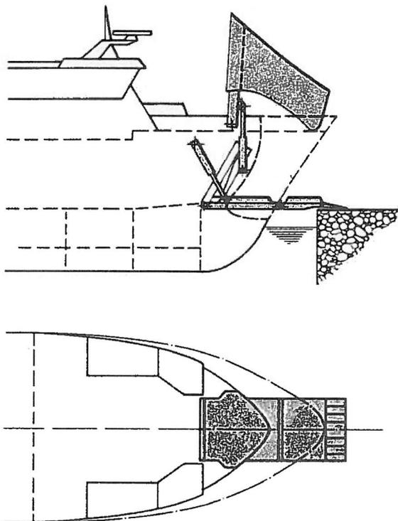
Above: The visor is a one-piece, perfectly matched portion of the ship's bow, hinged at forecastle (i.e. weatherdeck) level. The one shown above – on an 1,800grt car-passenger ferry, operating in the Adriatic – swings open to provide clearance for vehicles traversing the two-section 8.9m long x 4.2m wide bow ramp; this latter, when folded into stowage, doubles as a watertight door, being forced against a compression seal by hydraulically operated cleats.
