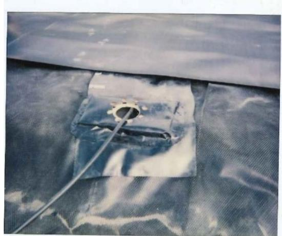
Exhibit 2-6: Leak detection test (July 11, 1992)
