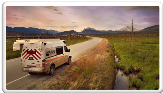
Figure 9: Pavement Data Collection Van Located on the Dalton Highway.
