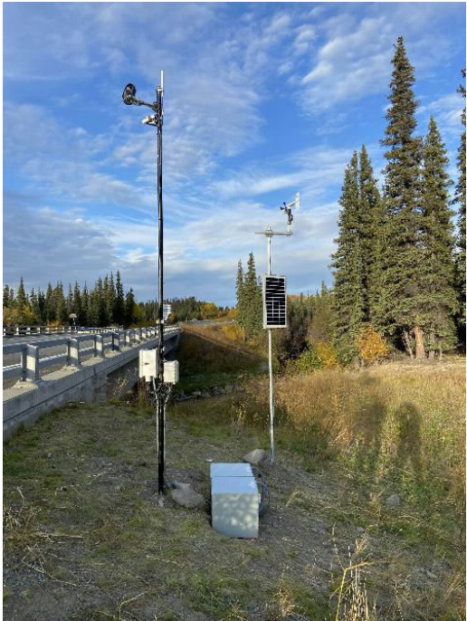
Photo Credit: "Alicia Stevens, DOT&PF" Description: Mini RWIS station located at MP17 of the Tok Cutoff, installed for a pilot project in 2021.
