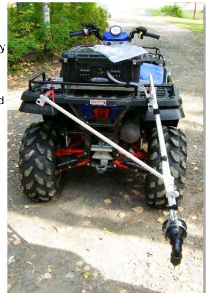
Pictured: The DUSTM—a portable, versatile instrument that can attach to an ATV.
