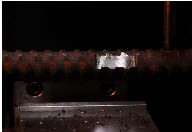
Figure 4.22 Rebar after Milling
