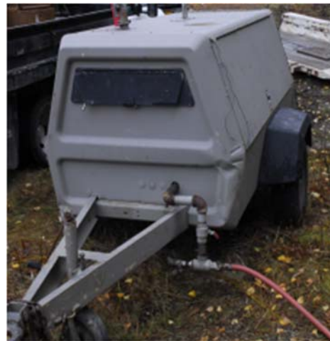
(b) Air Compressor
