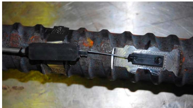
Figure 4.24 Rebar with Welded HPI Strain Gage
