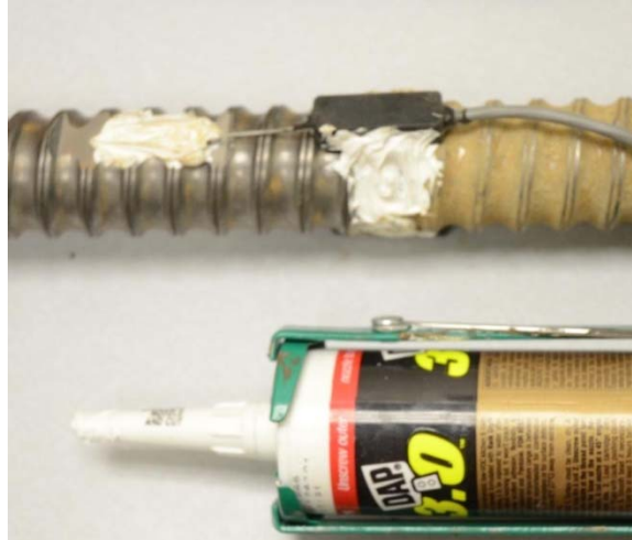
Figure 4.25 HPI Strain Gage with Silicone Caulk Protection
