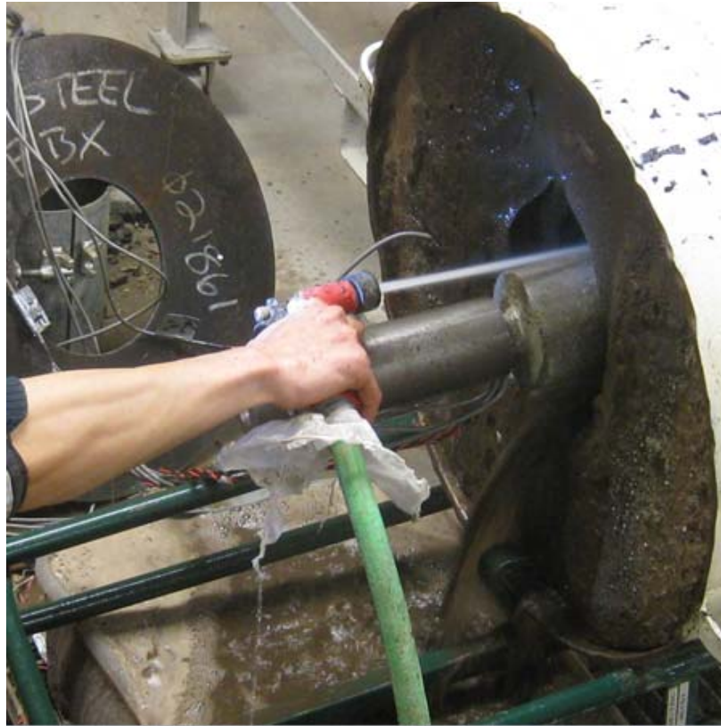
Figure 3.11 Oversize Hole before Installation of Grouted Anchor
