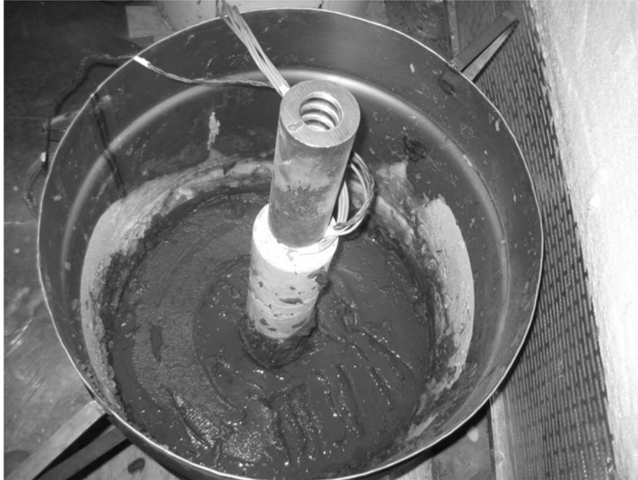
Figure 3.10 Layered Installation Method for Grouted Anchor
