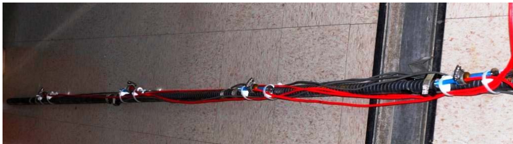
Figure 4.28 Anchor Bar with All Sensors
