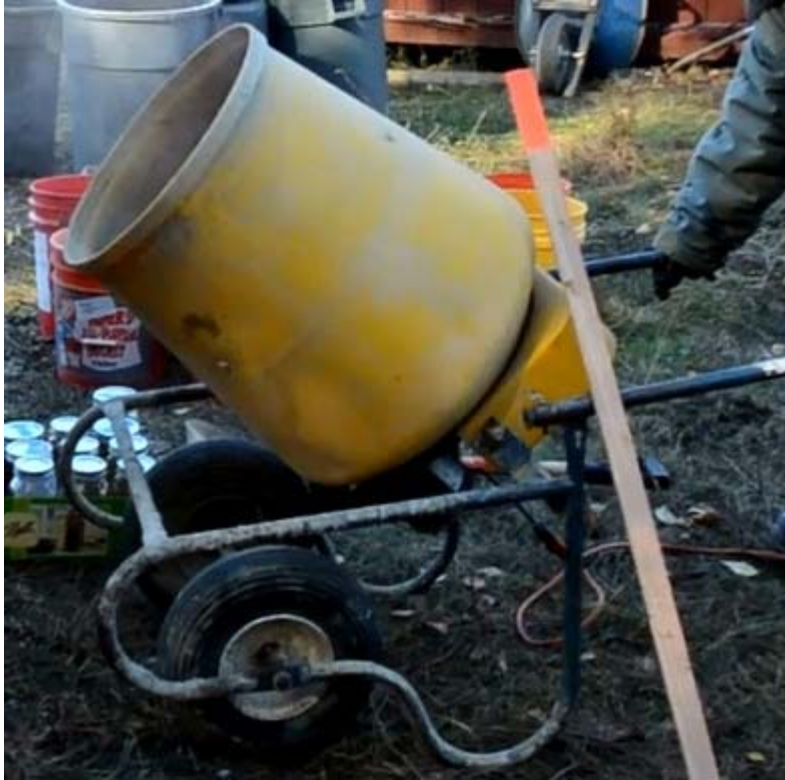
Figure 4.32 Backfill Material Mixing Equipment 2
