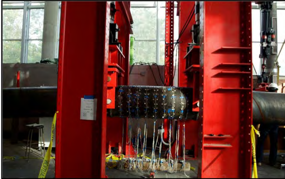
Figure 3-176: Specimen at maximum ductility displacement, ductility 4, \Delta = 8.0 inches
