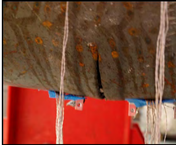
Figure 3-119: Second steel pipe rupture, Ductility 6, \Delta=9.67 in
