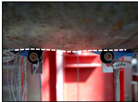
Figure 3-106: Pile buckle, Ductility 2-1st pull, \Delta=3.3 in
