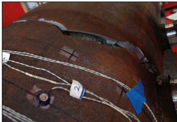
Figure 3-77: Rupture of the steel pipe during the first pull of ductility seven
