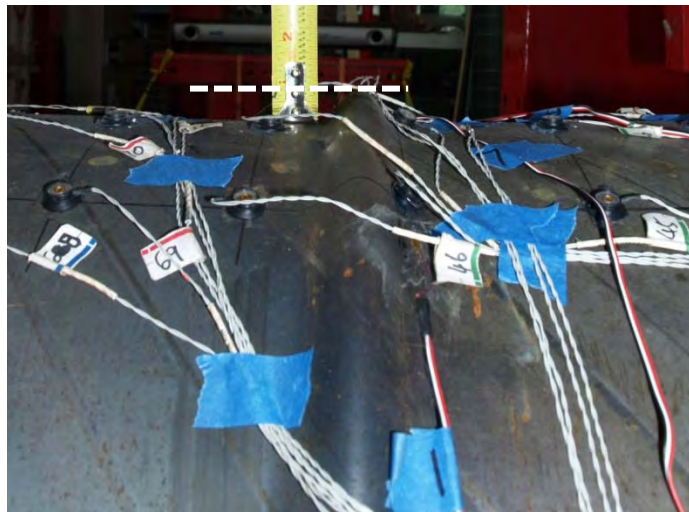
Figure 3-96: Buckle on top of pile, Ductility 5, \Delta = 9.4 in
