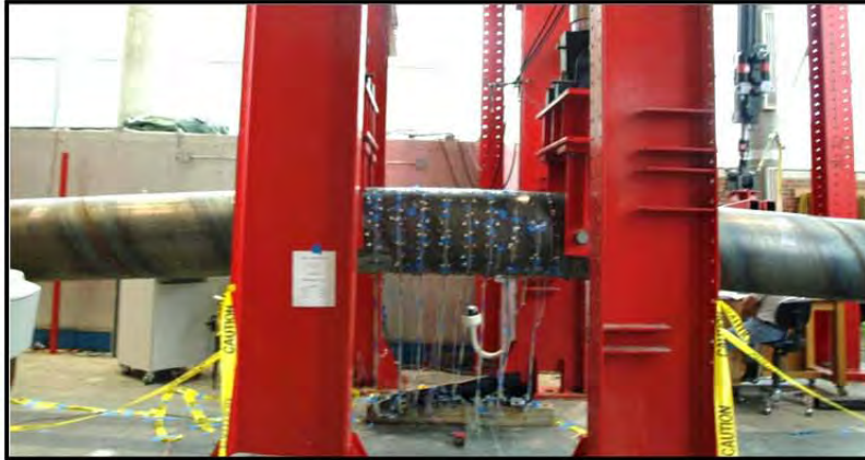
Figure 3-136: Displaced pile profile, ductility 4, \Delta=11.2 inches
