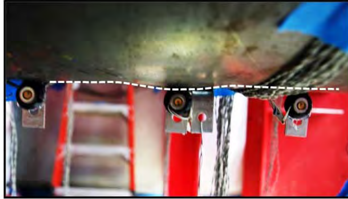
Figure 3-103: Initiation of buckling, Ductility 1-3rd pull, \Delta = 1.67 in
