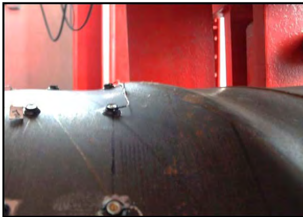
Figure 3-200: Buckle near loading point, ductility 3, \Delta=6.6 in
