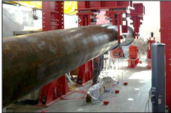
Figure 3-49: Pile profile at ductility five ( \Delta = 15 inches)
