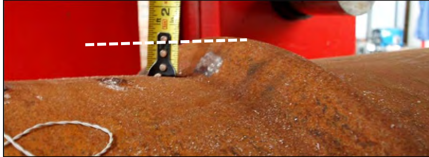
Figure 3-60: Size of buckle at ductility 4, \Delta = 13.1 inches
