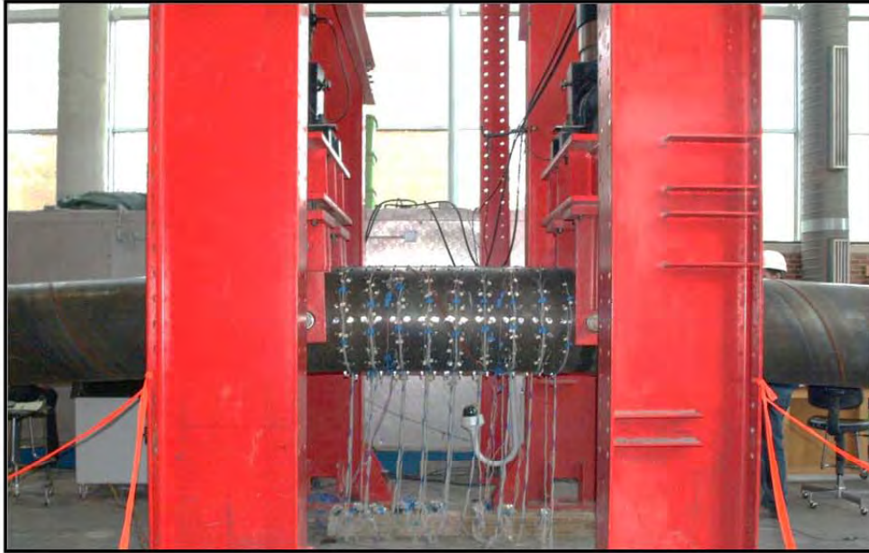
Figure 3-197: Deformed specimen, ductility 3, \Delta=6.6 in
