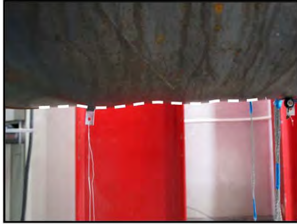
Figure 3-172: Ripples on steel pile, ductility 3 – 1st pull, \Delta = 6.0 inches
