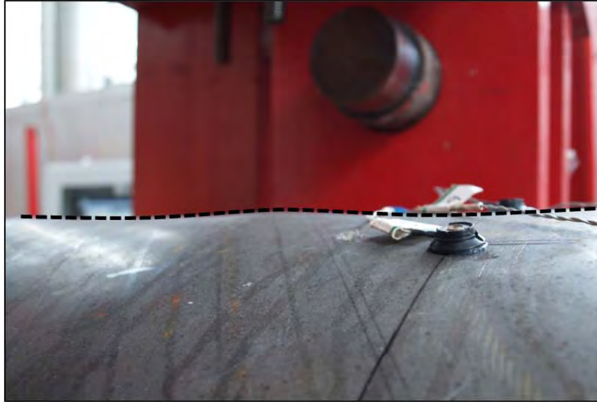
Figure 3-85: “Ripple” under loading point, Ductility 2, \Delta=3.8\text{in}
