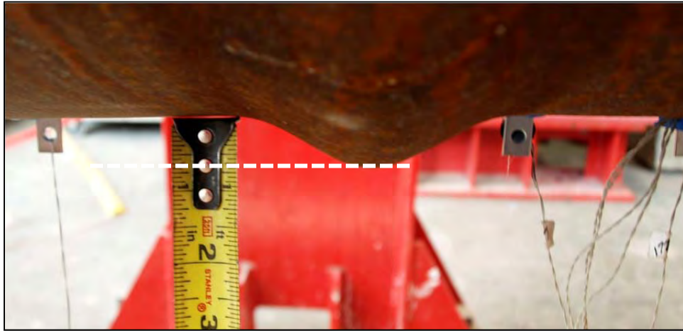
Figure 3-56: Buckle under loading point, ductility 3, \Delta = 9.8 inches
