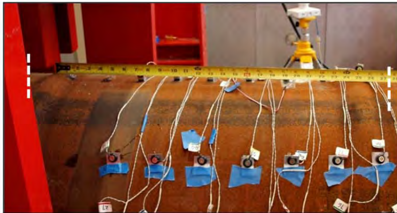
Figure 3-59: Spacing of buckles at ductility 3, \Delta = 9.8 inches
