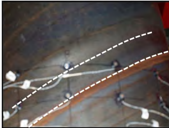
Figure 3-177: Buckle following weld direction, ductility 4, \Delta = 8.0 inches
