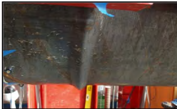
Figure 3-155: Buckle under the loading point, spreading half the circumference of the specimen, ductility 3, \Delta=6.9 inches
