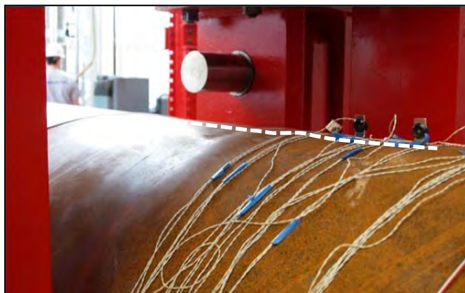
Figure 3-36: Visible signs of buckling under the actuator at ductility 3, displacement = 6.8 inches
