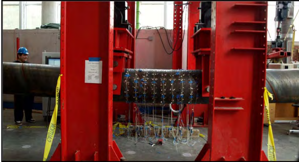
Figure 3-170: Pile profile, ductility 3, \Delta = 6.0 inches
