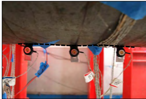
Figure 3-81: Initiation of buckling, Ductility 1.5 first pull, \Delta=1.8 inches
