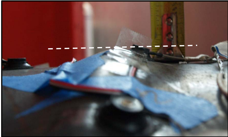
Figure 3-129: Buckle located between loading points, ductility 2, \Delta=5.7 in
