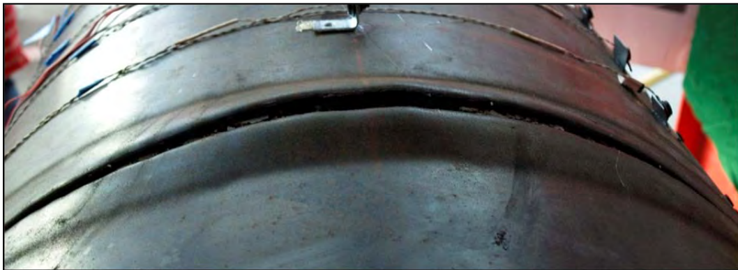
Figure 3-31: Rupture during the second pull of ductility six, at a displacement of 12.5 inches
