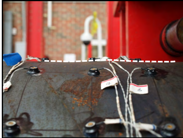
Figure 3-192: Initiation of buckling on top of pile, ductility 1.5, \Delta=3.3 in
