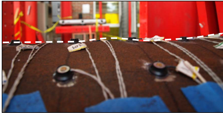
Figure 3-72: “Ripples” in the constant moment region, second push ductility six, \Delta = 15.6 in
