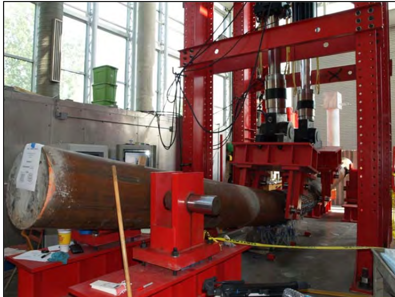
Figure 3-74: Pile profile with a mid-span displacement of 18.2 inches (ductility seven).
