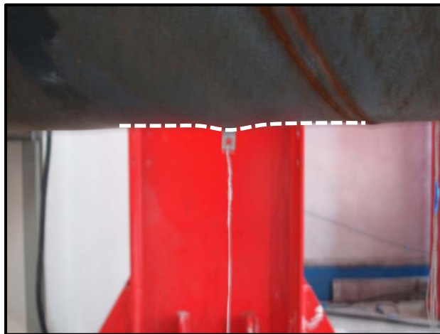
Figure 3-195: Ripple under the north loading point, ductility 2, \Delta=4.5 in
