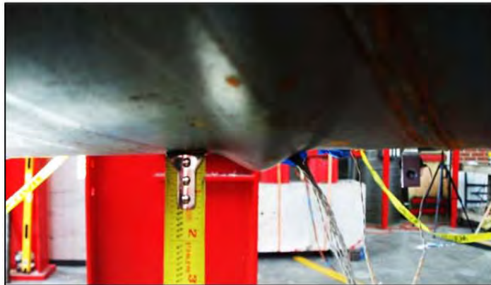
Figure 3-91: Buckles with a height of \frac{1}{2} inch, , Ductility 3, \Delta = 5.6 in
