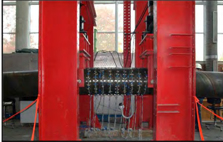
Figure 3-202: Deformed specimen, ductility 4, \Delta=8.9 in
