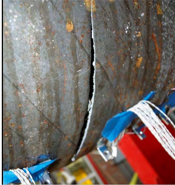
Figure 3-117: Steel pipe rupture, \Delta=8.40 in
