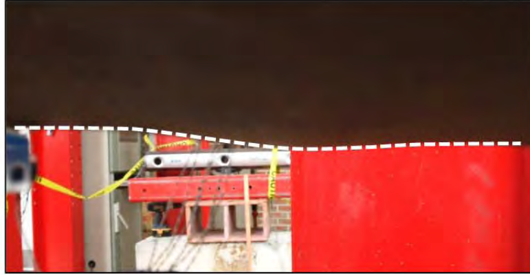
Figure 3-69: Buckle on the underside during ductility five, \Delta = 13 inches
