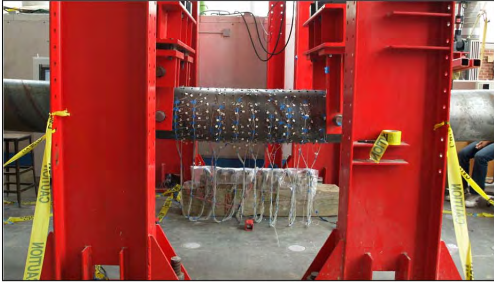
Figure 3-83: Specimen profile, Ductility 2, \Delta=3.8\text{in}
