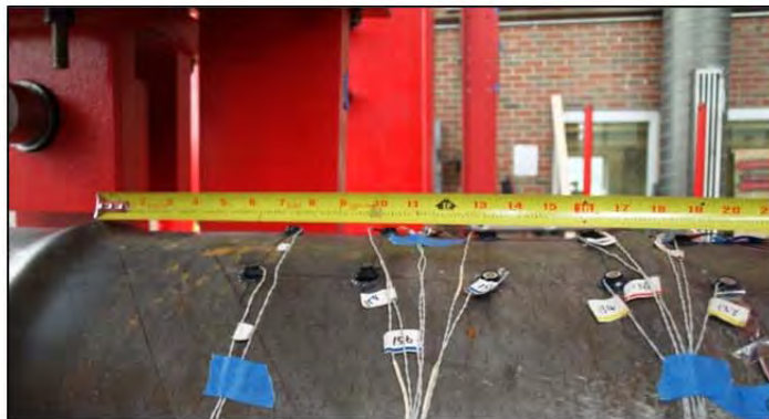
Figure 3-92: Buckles spaced evenly (17-20" apart), Ductility 3, \Delta = 5.6 in
