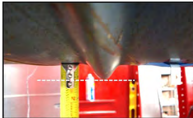
Figure 3-158: Buckle under loading point, ductility 4, \Delta=9.2 inches
