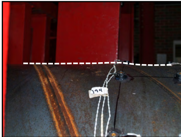
Figure 3-193: Typical buckle at the end of ductility 1.5, \Delta=3.3 in
