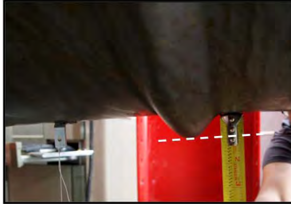
Figure 3-182: Buckle under loading point, ductility 5, \Delta = 10.0 inches
