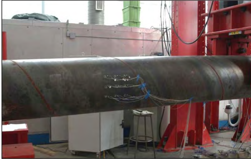
Figure 4-26 Photograph of the LED targets measuring the slip between the steel tube and concrete
