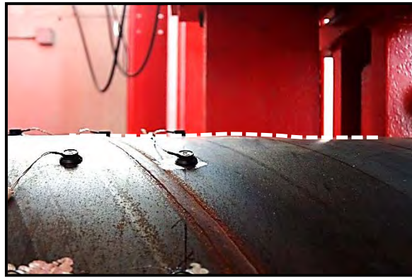
Figure 3-168: Initiation of buckling, ductility 2, \Delta = 4.0 inches
