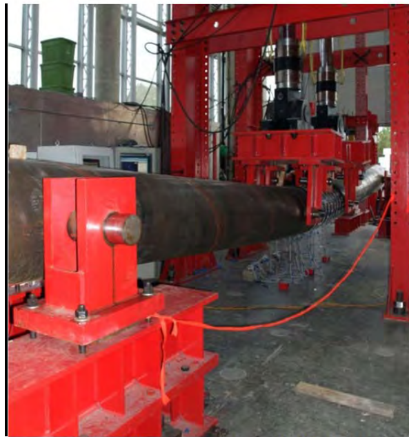
Figure 3-205: Deformed specimen, ductility 5, \Delta=11.1 in
