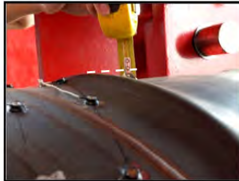
Figure 3-179: Buckle under loading point, ductility 4, \Delta = 8.0 inches
