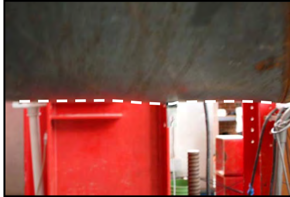
Figure 3-169: Initiation of buckling, ductility 2, \Delta = 4.0 inches
