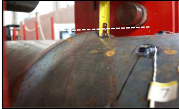
Figure 3-153: Buckle under loading point, ductility 3, \Delta=6.9 inches
