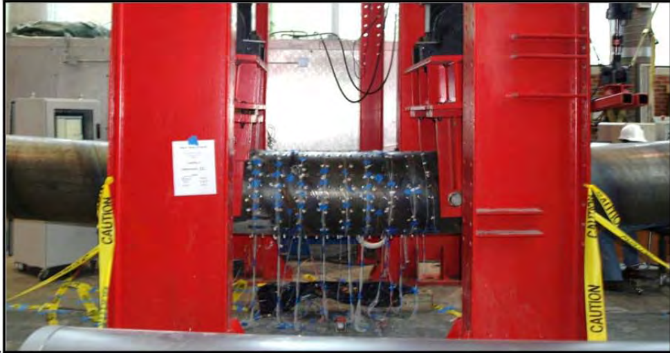
Figure 3-131; Displaced pile profile, ductility 3, \Delta=8.4 inches
