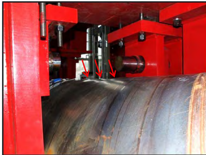
Figure 3-198: Ripples on top of pile, ductility 3-push 1, \Delta=6.6 in
