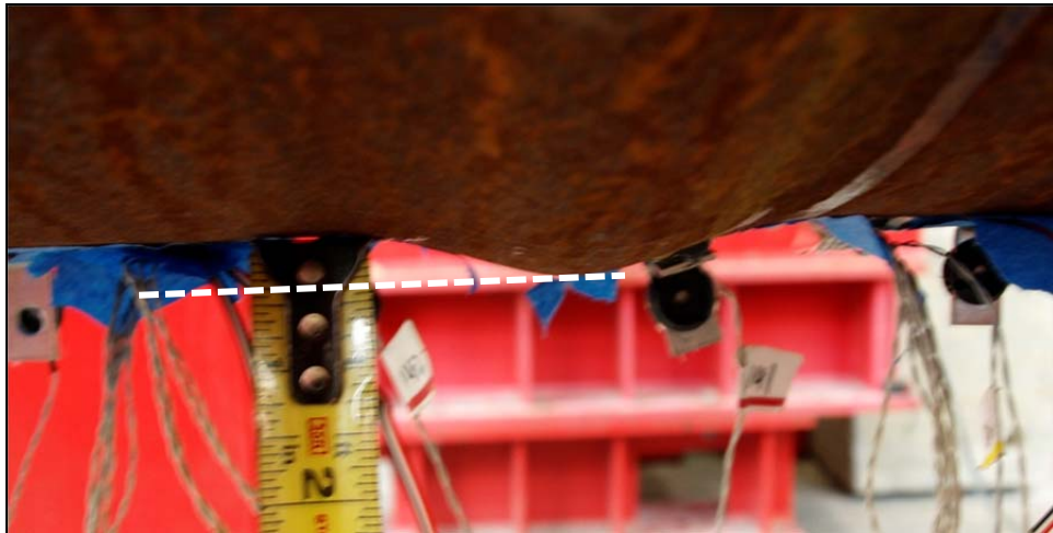
Figure 3-57: Buckle in constant moment region, ductility 3, \Delta = 9.8 inches
