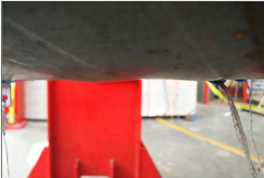
Figure 3-86: “Ripples” under loading point, Ductility 2, \Delta=3.8\text{in}
