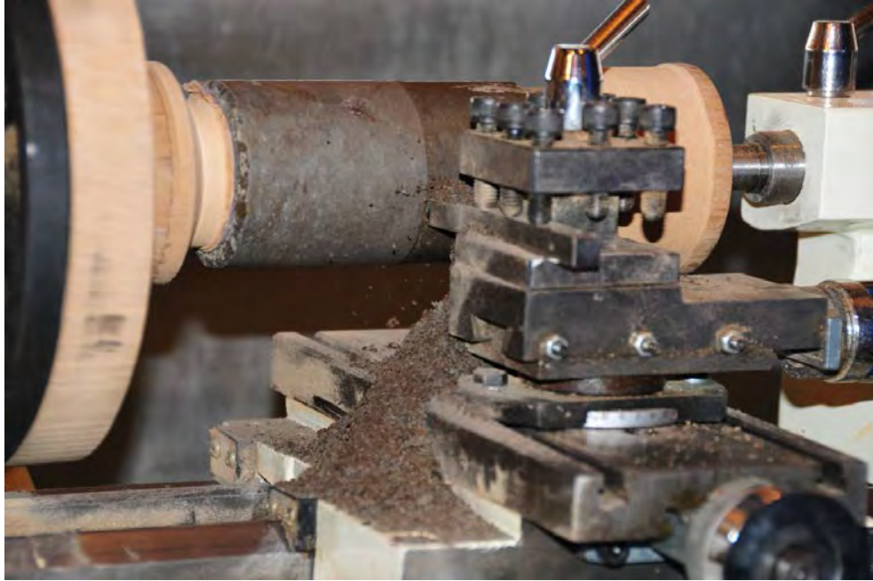
Figure 2.4 A frozen soil specimen in the special holding bit on the lathe.
