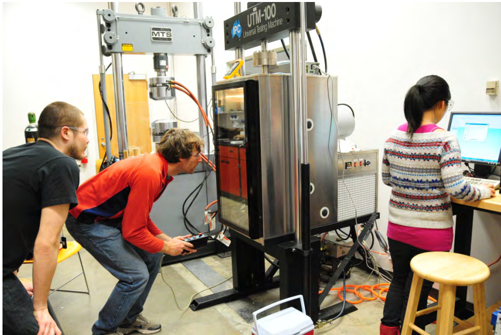
Figure 2.8 The Universal Testing Machine (UTM-100) with a temperature chamber and computer interface.
