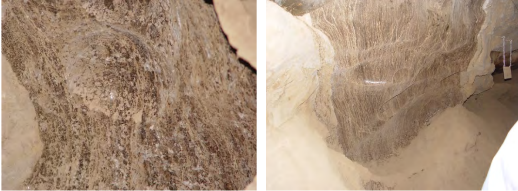
Figure 4.3 Ice wedges observed in the CRREL Permafrost Tunnel.
