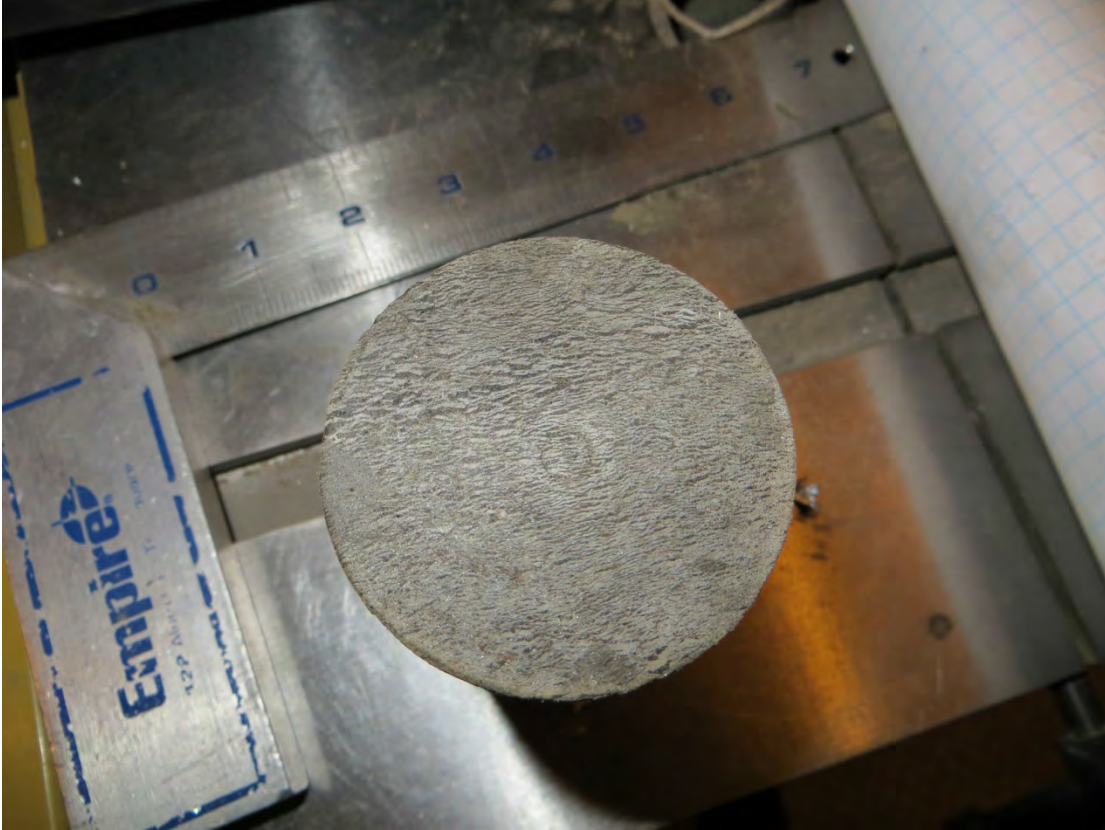
Figure 3.7 Specimen P4 H4 with small defect at the center of one end.
