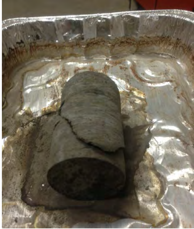
Figure 3.11 Failure of specimen P4 V2 due to shearing.
