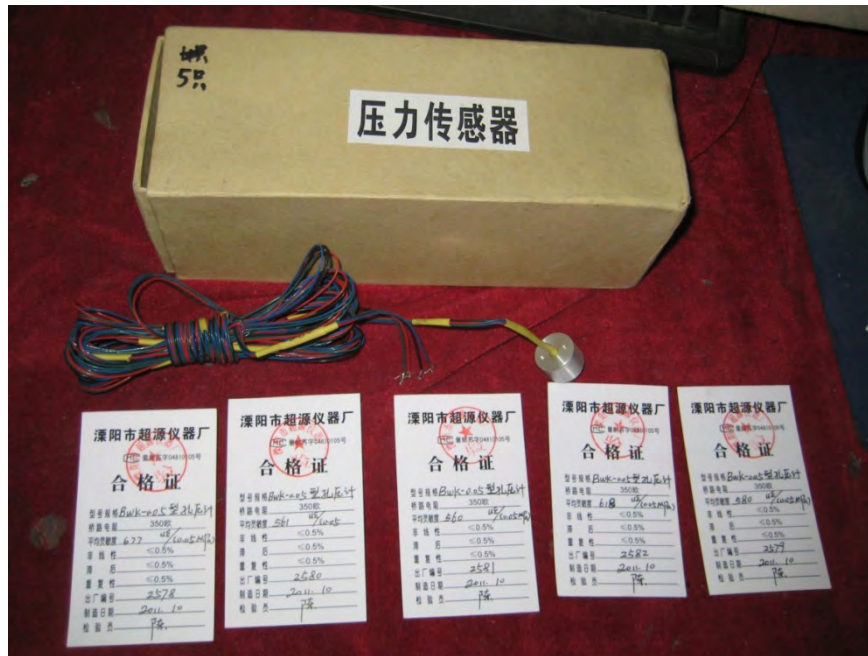
Figure 2.10. Pore pressure sensors
