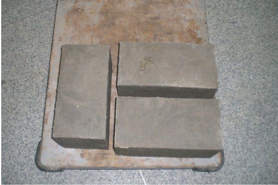
Figure 2.4. Cemented sand specimens
