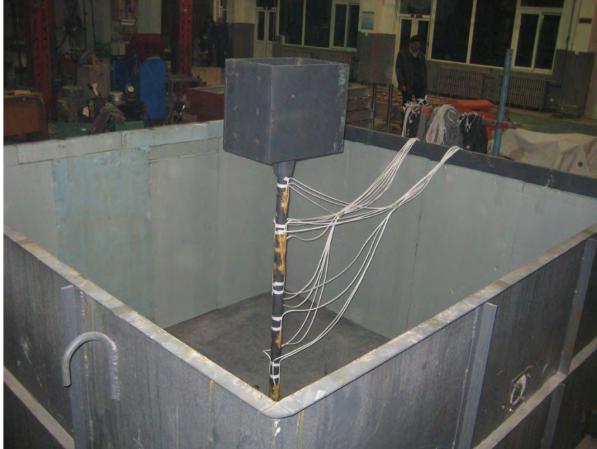
Figure 2.7. Soil box and pile with strain gauges installed and wired
