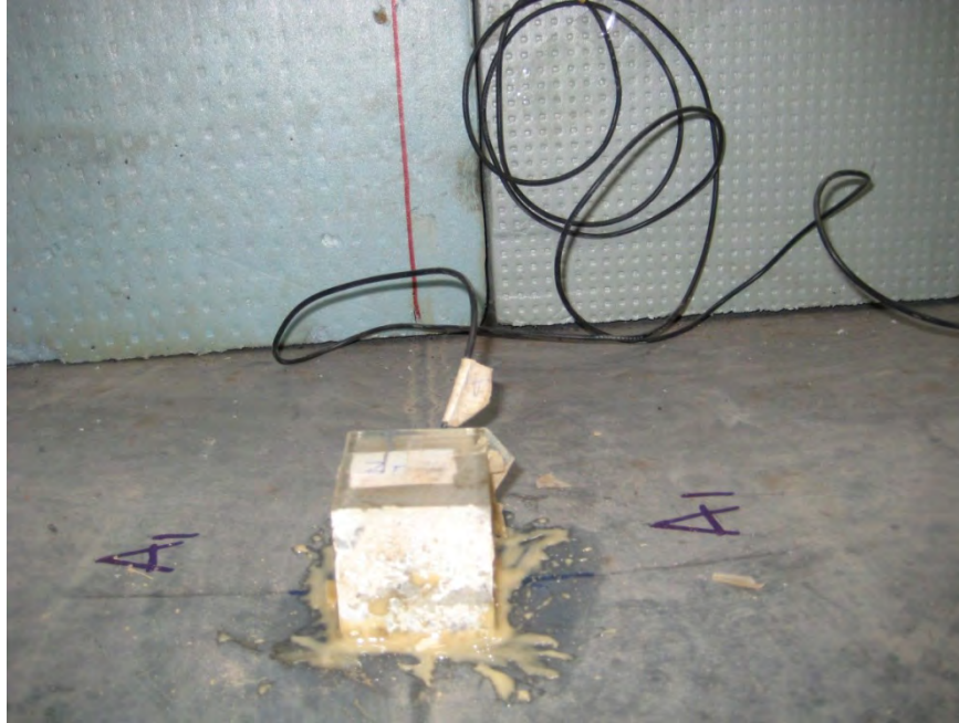
Figure 2.12. An accelerometer in a waterproof enclosure as installed on the bottom of the soil container
