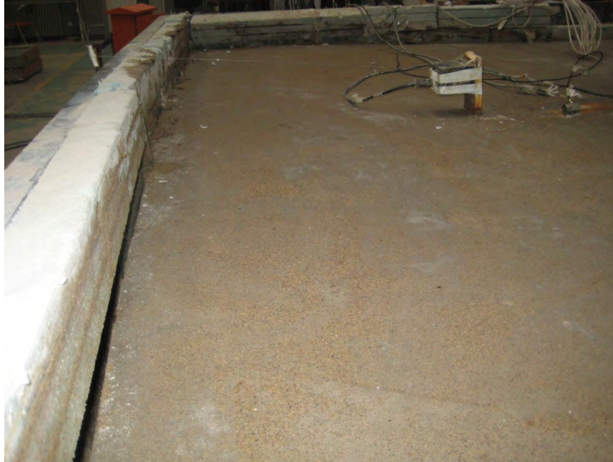
Figure 2.18. Lateral spreading of the simulated frozen crust
