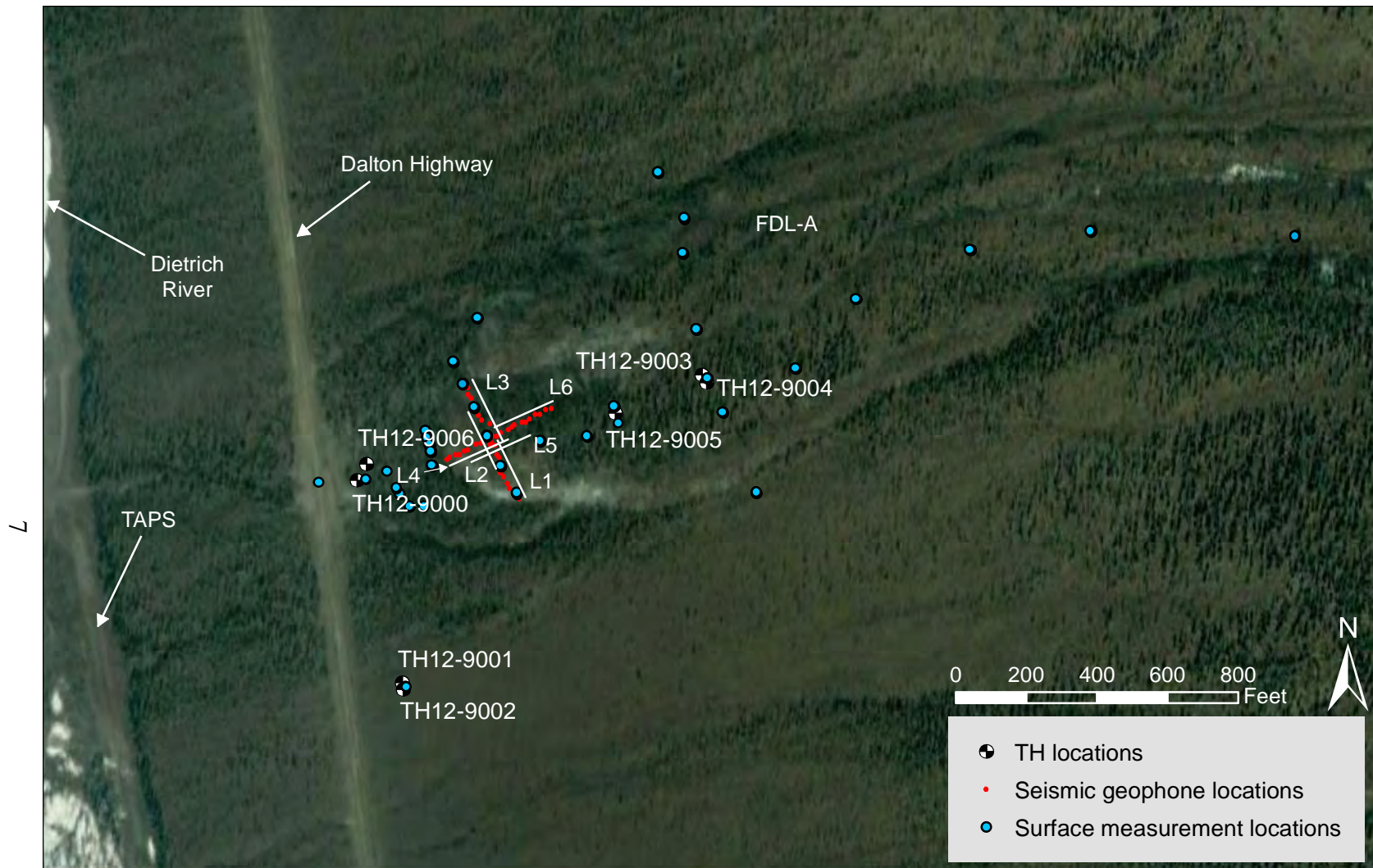
Figure 5. Locations of field measurements on and near FDL-A. The base image, which was imported from Google Earth, was acquired in 2002. It does not accurately represent the location of FDL-A, which has advanced since its acquisition. Currently the toe of the lobe is at the location of the blue surface measurement points that intersect the text of “TH12-9000”. The placement of the seismic lines is represented by white lines adjacent to the geophone locations.
