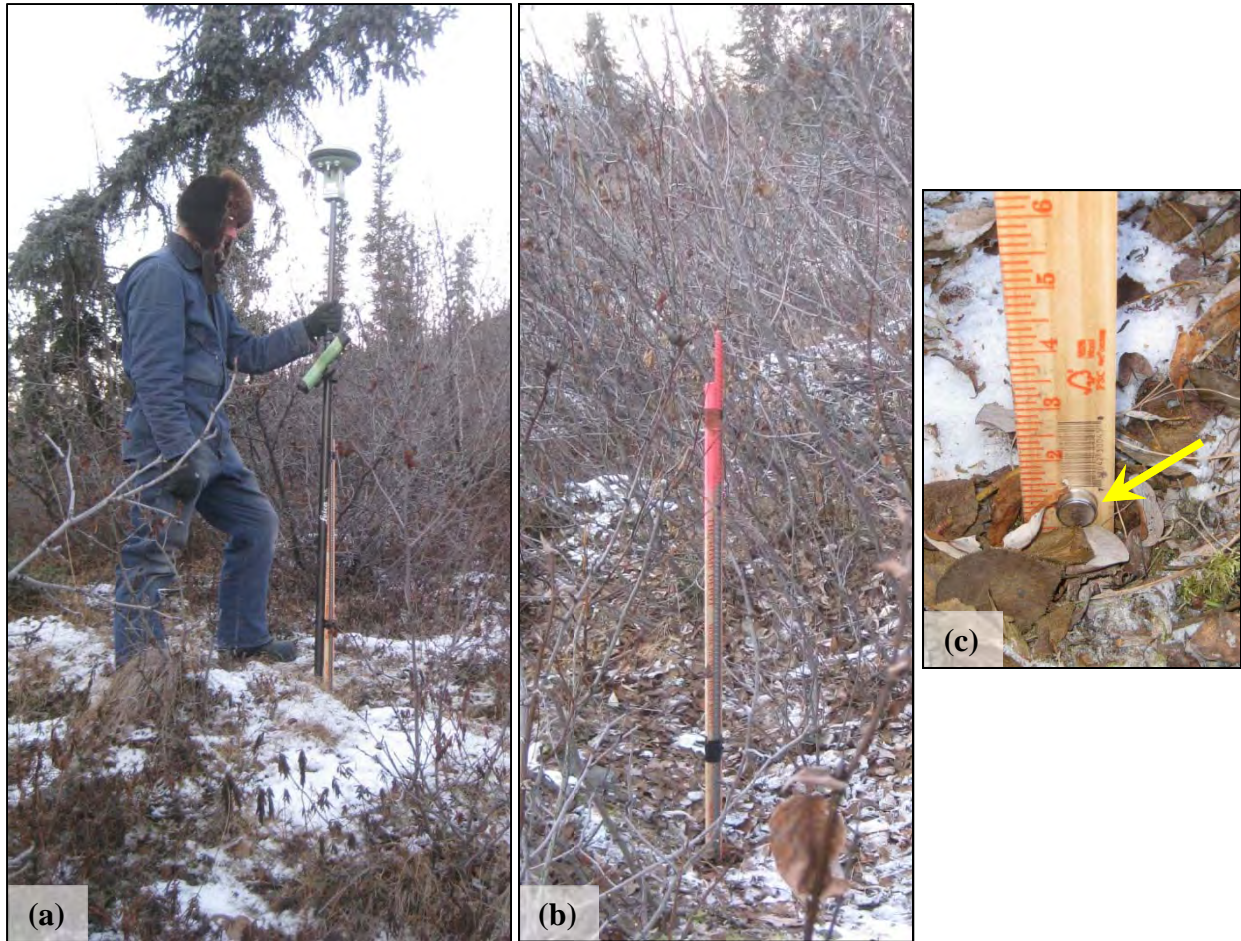
Figure 15. Measuring movement of the FDL-A surface. (a) Repeated measurements were made throughout the fall using a differential global positioning system (D-GPS) unit. (b) We installed steel rods, with yard sticks (spray-painted pink for high visibility) and (c) temperature recording devices attached (indicated with yellow arrow). (Photographs by M. Darrow)
