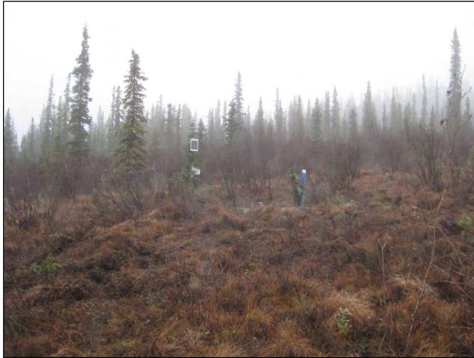
Figure B-5. Final set-up of the “undisturbed” satellite ADAS. This photograph was taken to the north; the Dalton Highway is located to the left of this photograph, and FDL-A is beyond the trees that are just visible in the fog. The ADAS and slotted casing were covered with tree branches to reduce their visibility from the highway. (Photograph by M. Darrow)
