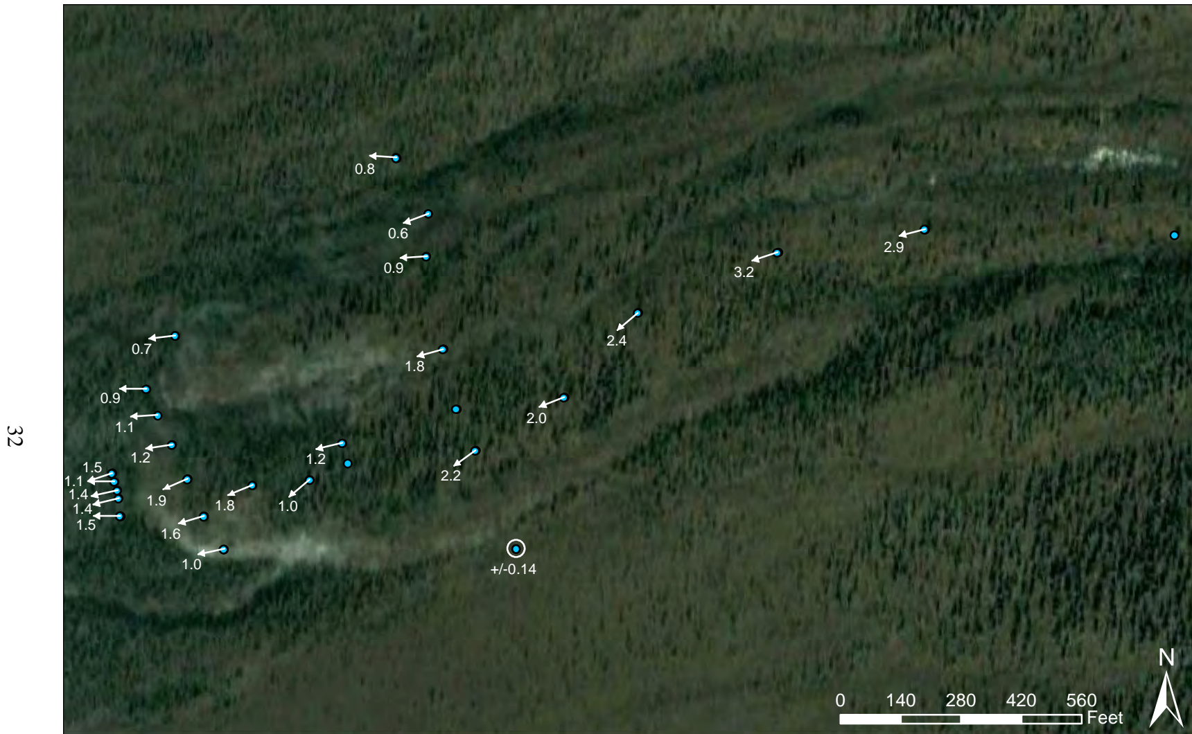
Figure 28. Summary of surface movement measurements. All points were measured using a differential global positioning system (DGPS). The length of all arrows is the same; they indicate direction of movement only, not velocity. Total movement for each point is provided in feet near the head of each arrow. The circle around the southernmost point indicates the use of this point for error calculations, which we estimate at +/-0.14 ft.
