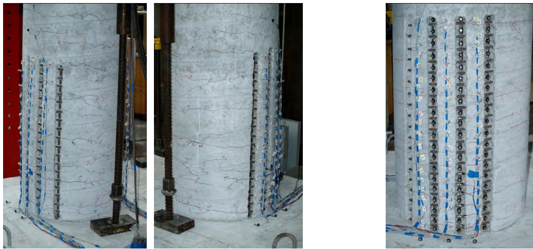
Figure 2-9. Test 9 – (Left) Front and Back of Specimen during ( \mu_2^{+1} = 1.69'' ) and (Right) South Crack Pattern during ( \mu_2^{-1} = -1.68'' )
