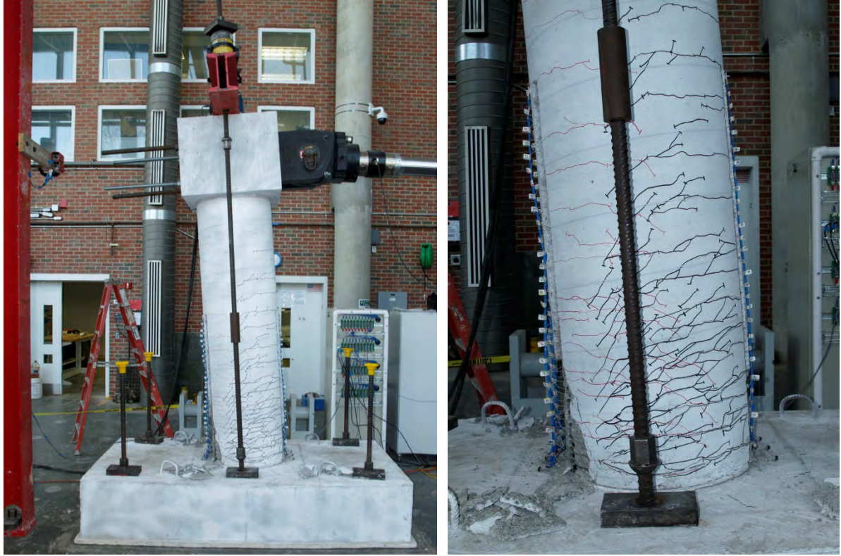
Figure 2-350. Test 18 – Crack Distribution at Peak Displacement ( \mu_{9,0}^{24.40 \text{ sec}} = 7.46'' )
