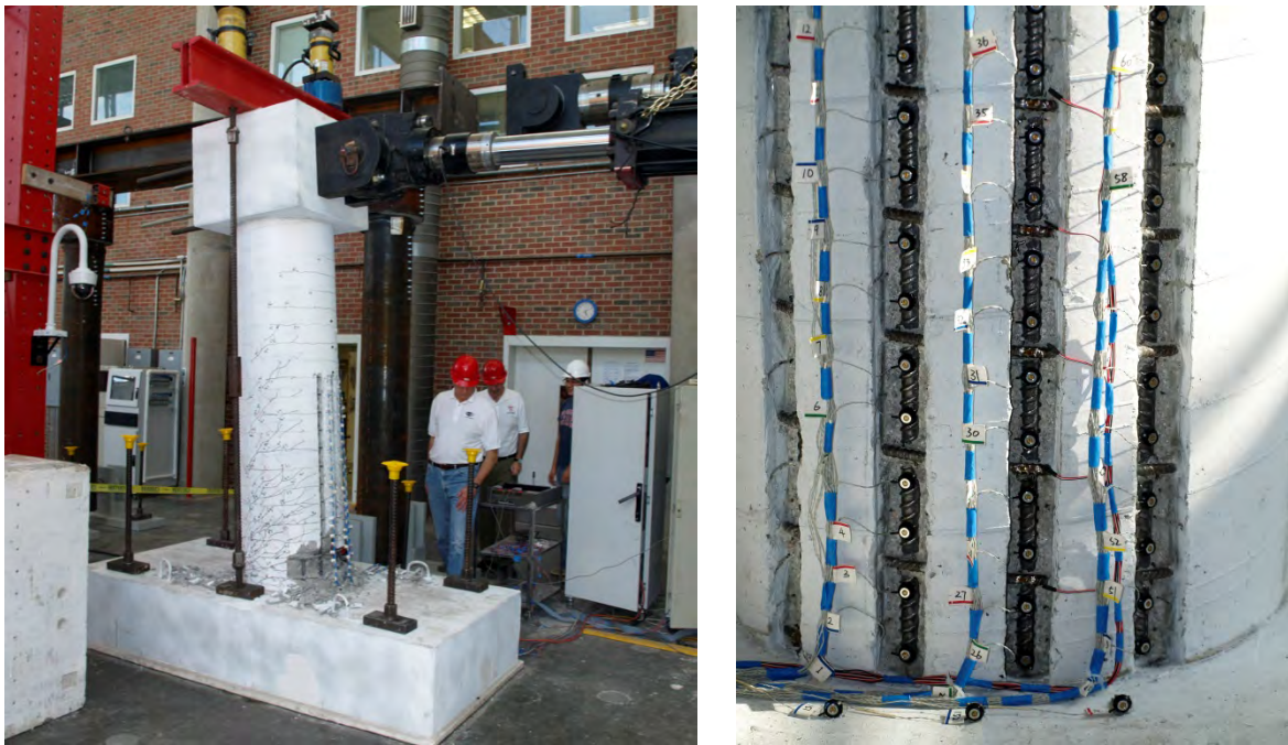
Figure 2-198. Test 14 – (Left) Test Setup and Specimen at ( \mu_8^{+2} = 6.40'' ) and (Right) Two Target Markers within Each 4" Transverse Steel Spacing
