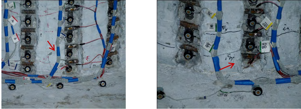
Figure 2-8. Test 9 – First Signs of Cover Concrete Flaking which Precedes Crushing (Left) South Side during ( \mu_2^{+2} = 1.69'' ) and (Right) North Side during ( \mu_2^{-2} = -1.67'' )
