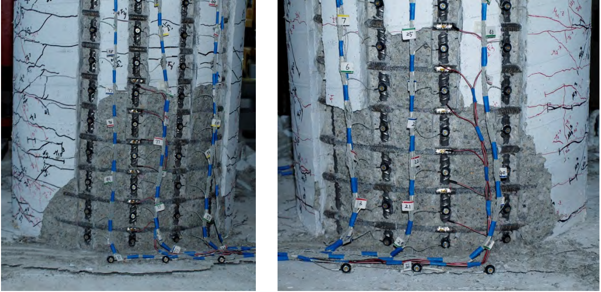
Figure 2-166. Test 13 – Extent of Crushing at the End of Ductility Six (Left - North) and (Right - South)
