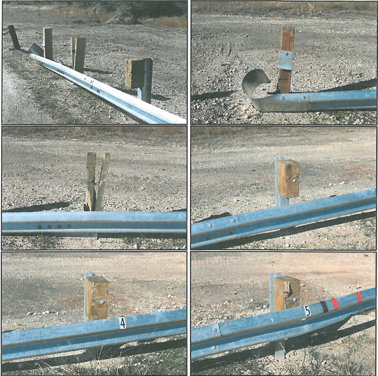
Figure 7.4. Posts 1 through 5 after Test No. 608331-01-6.
