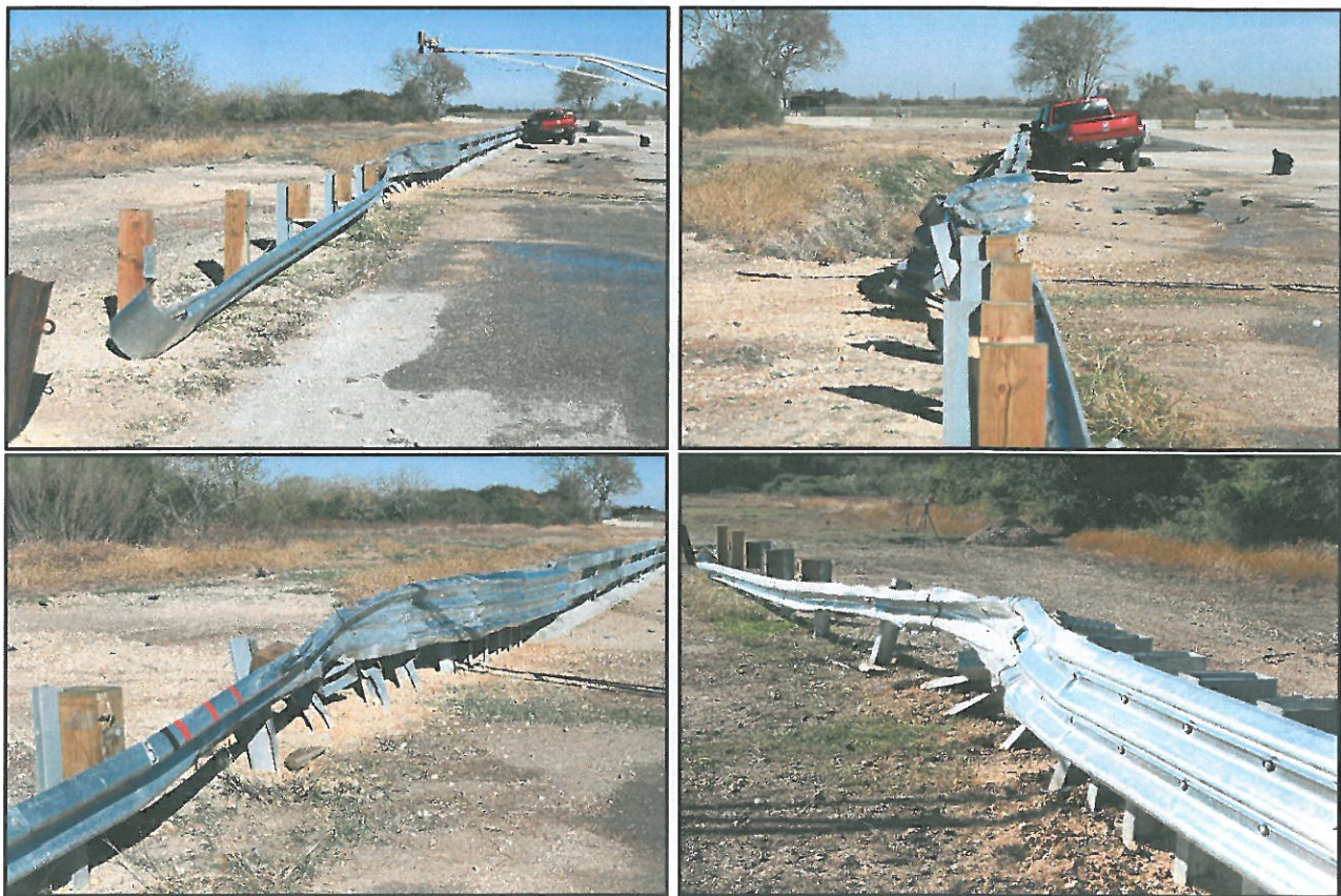
Figure 7.3. Transition after Test No. 608331-01-6.
