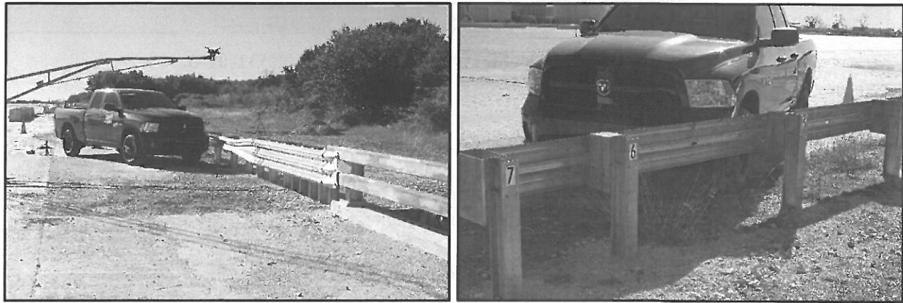
Figure 7.1. Transition/Test Vehicle Geometries for Test No. 608331-01-6.
