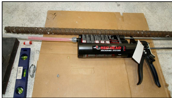
Figure 5.4: Redhead two-part epoxy application system
