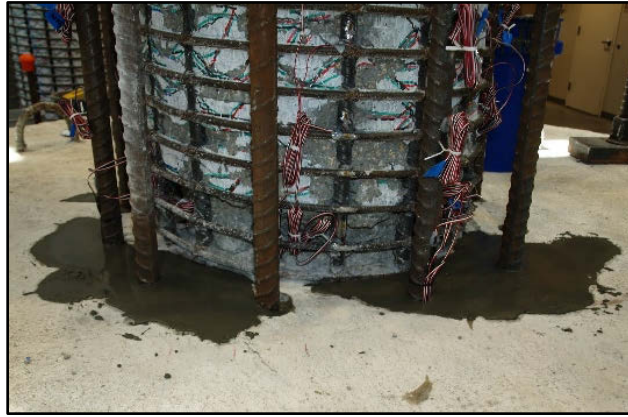
Figure 5.7: Installation of patch grout on top of footing
