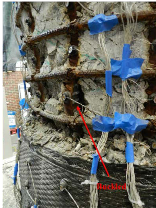
Figure 5.60 : Damage During \mu_{4\Delta}
