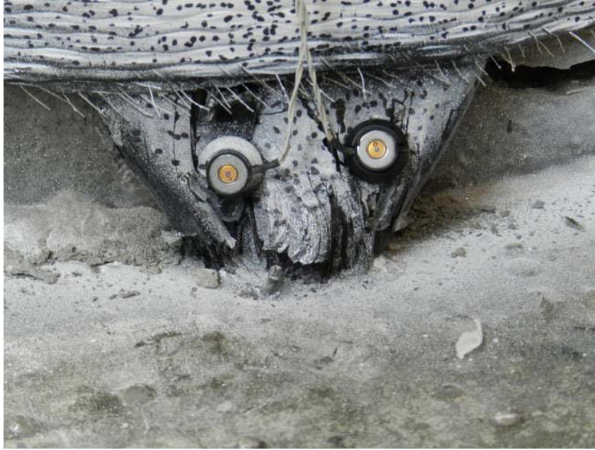
Figure 4.23: Fiber Rupture in the CF Anchor
