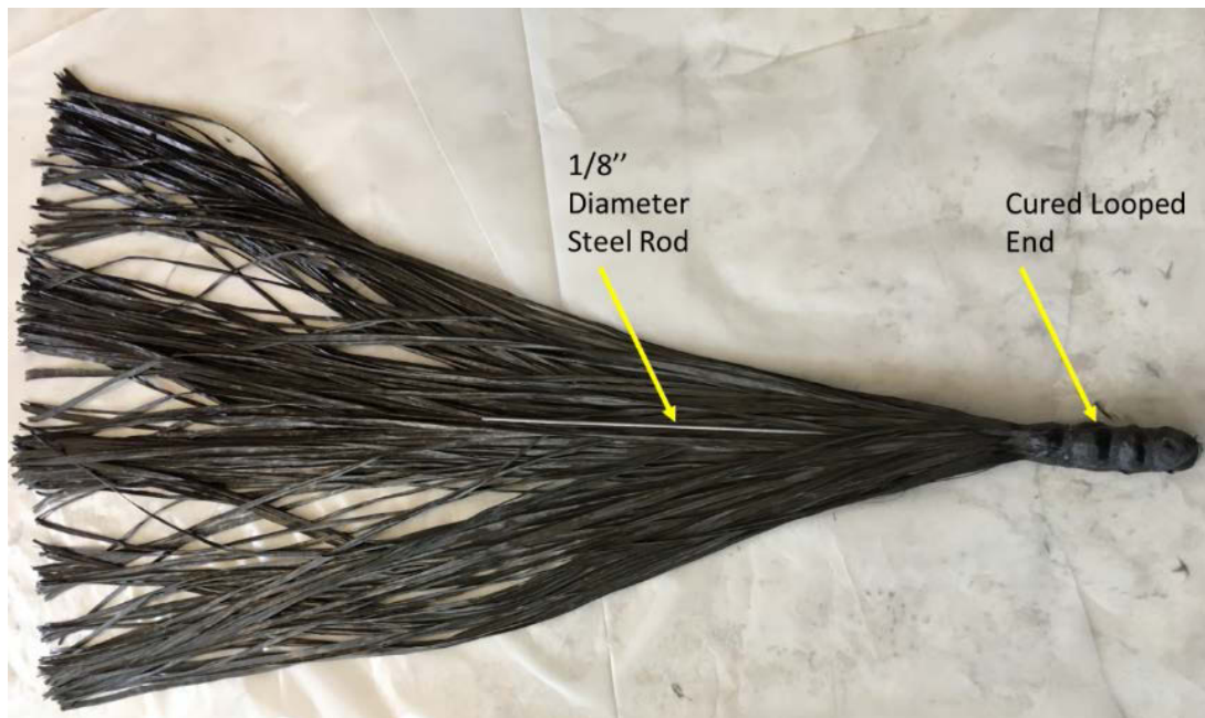
Figure 5.21: Preparation of Anchor Ends
