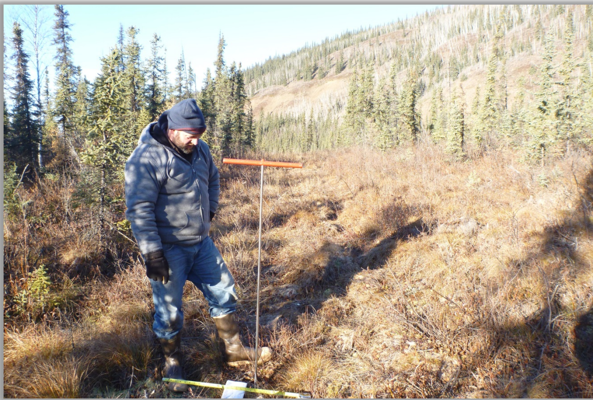
Figure 19. Active layer probing in center of winter trail near Monitoring Station # 1.
