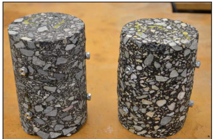
Samples before and after the flow number (FN) test. This procedure was derived from AASHTO TP 79-13. The FN test is used to evaluate the creep characteristics of HMA and results in permanent deformation of the test specimen.
