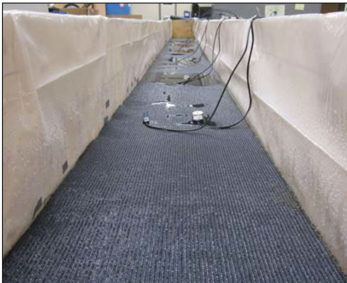
One set of sensors was put at each location, and 8 sets of sensors were put in one layer. The fabric was then saturated with water before another layer of soil was put into the testing flume.
