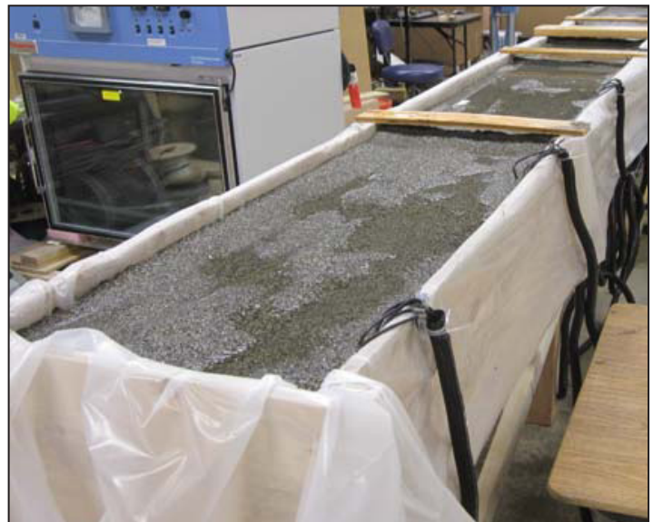
The testing flume filled with 12 in. of saturated sand.
