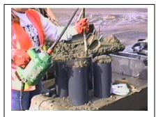
Vibrating cylinder specimens
