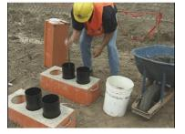
Consolidation of concrete in cylinder by rodding
