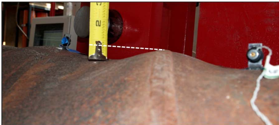
Figure 3-22: Buckling under north loading point at ductility 5 push 1, at a displacement of 17.07 inches
