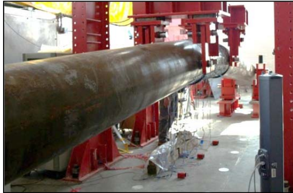
Figure 3-49: Pile profile at ductility five ( \Delta = 15 inches)
