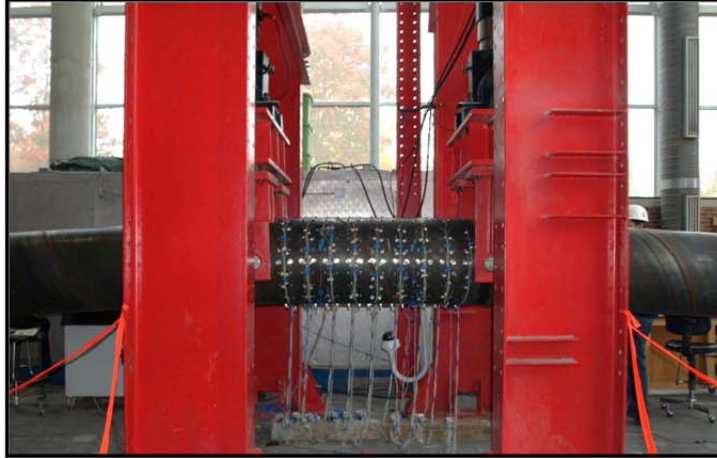
Figure 3-202: Deformed specimen, ductility 4, \Delta=8.9 in
