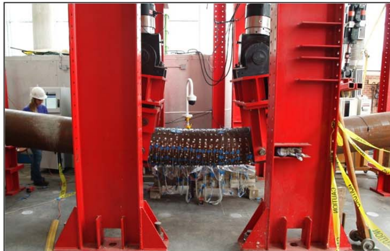
Figure 3-70: Pile profile with a mid-span displacement of 15.6 inches (ductility six)
