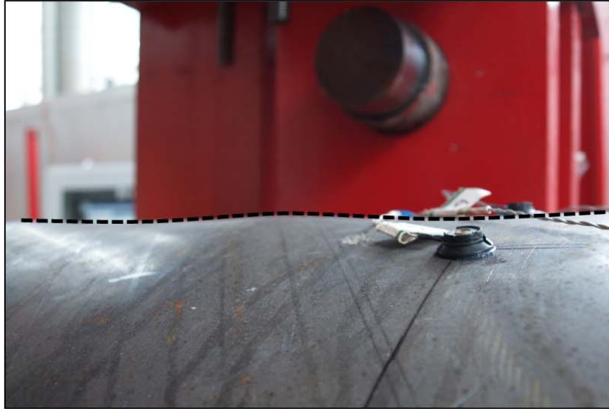
Figure 3-85: “Ripple” under loading point, Ductility 2, \Delta=3.8\text{in}
