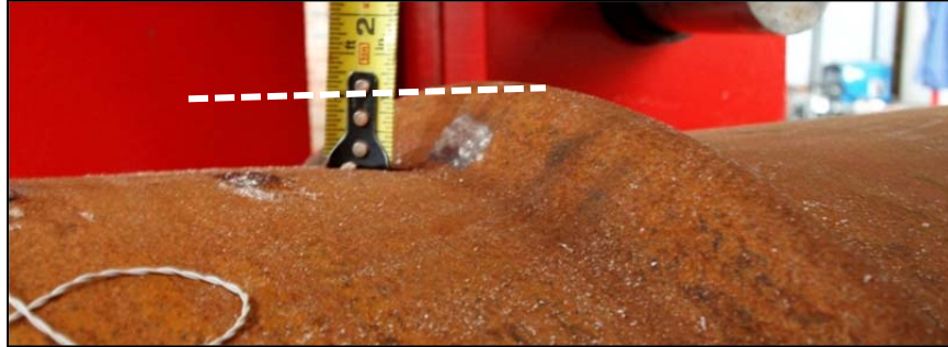
Figure 3-60: Size of buckle at ductility 4, \Delta = 13.1 inches
