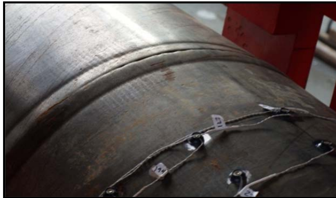
Figure 3-163: Rupture on top of the pile, first pull of ductility 5, \Delta=11.5 in
