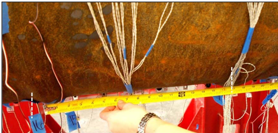
Figure 3-38: Buckles spaced 18-20" at ductility 4, displacement = 8.4 inches
