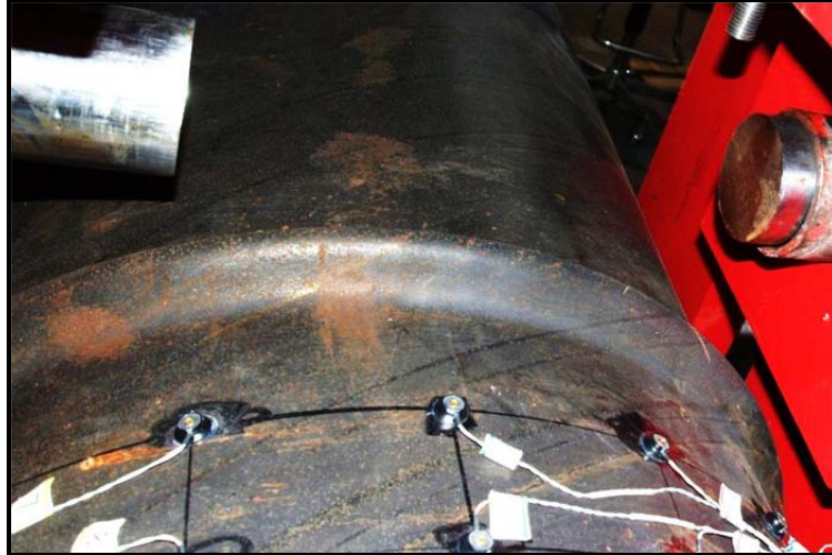
Figure 3-208: Narrow buckle on the top of the pile under loading point, ductility 5, \Delta=11.1 in
