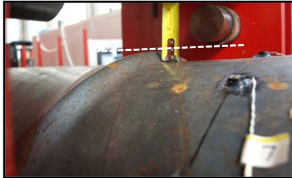
Figure 3-153: Buckle under loading point, ductility 3, \Delta=6.9 inches
