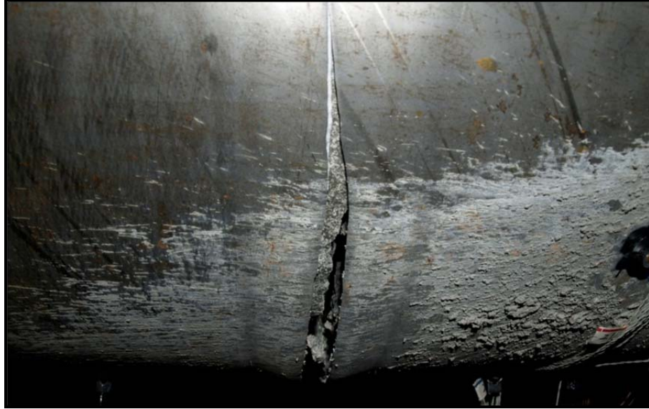
Figure 3-140: Rupture on the underside of the pile at full displacement of ductility 4, \Delta=11.2 in
