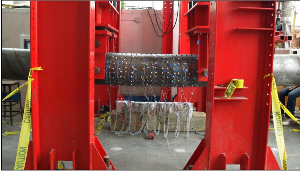
Figure 3-83: Specimen profile, Ductility 2, \Delta=3.8\text{in}
