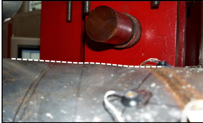
Figure 3-125: Initiation of buckling, Ductility 1-2nd push, \Delta = 2.80 in
