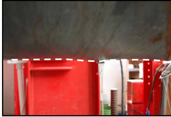
Figure 3-169: Initiation of buckling, ductility 2, \Delta = 4.0 inches
