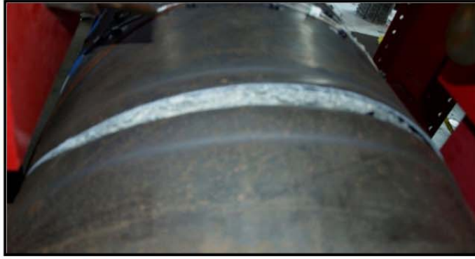
Figure 3-187: Rupture of the steel pile, ductility 6, \Delta=12 inches
