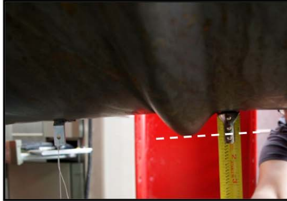
Figure 3-182: Buckle under loading point, ductility 5, \Delta = 10.0 inches
