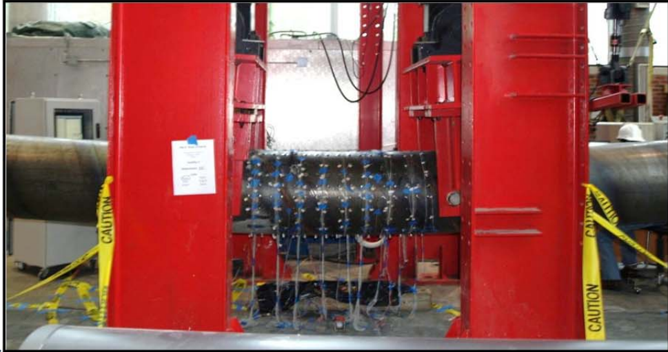
Figure 3-131; Displaced pile profile, ductility 3, \Delta=8.4 inches
