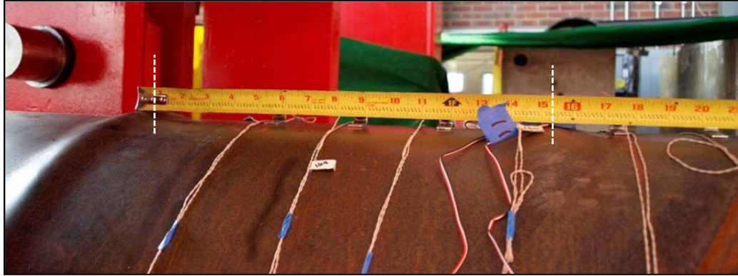
Figure 3-28: Ductility 3 Push 1, buckles spaced 16-20 inches
