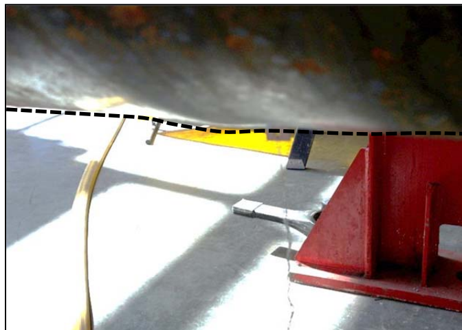
Figure 3-27: Ductility 1.5 – first signs of buckling
