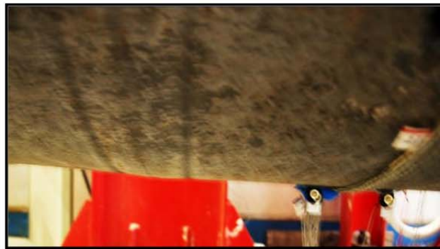
Figure 3-137: Tension cracks observed on the underside of the pile, ductility 4, \Delta=11.2 in
