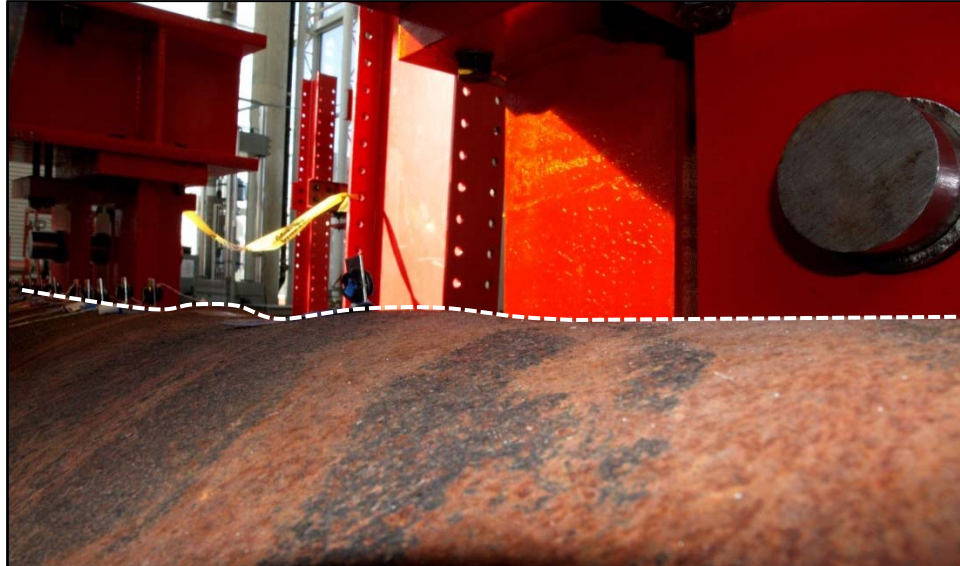
Figure 3-20: First signs of buckling at ductility 4 push 1, 13.67 inch displacement.
