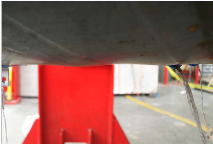
Figure 3-86: “Ripples” under loading point, Ductility 2, \Delta=3.8\text{in}
