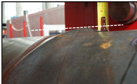
Figure 3-150: Buckle under loading point at ductility 2, \Delta = 4.6 inches
