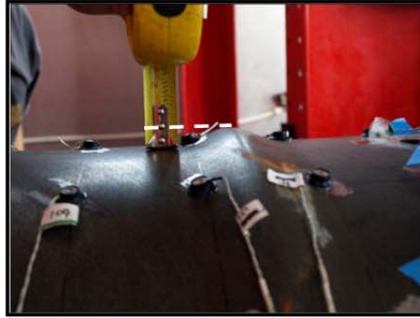
Figure 3-180: Buckle in constant moment region, ductility 4, \Delta = 8.0 inches
