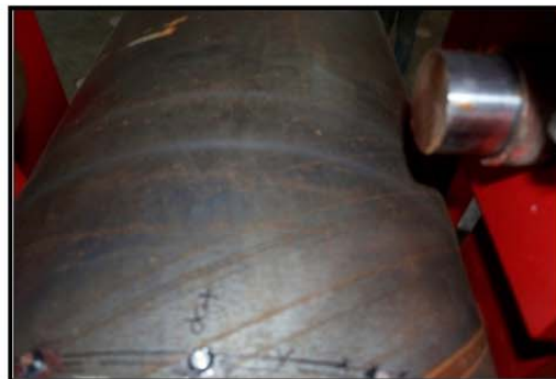
Figure 3-184: Tension cracks on the top of the pile, ductility 5, \Delta = 10.0 in
