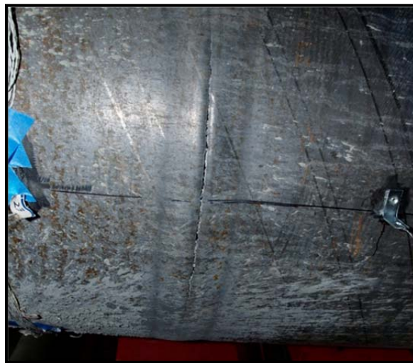
Figure 3-139: Rupture on the underside of the pile, during the first push of ductility 4
