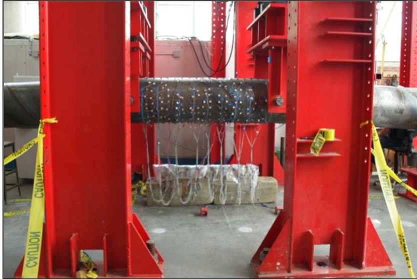
Figure 3-88: Pile profile, Ductility 3, \Delta = 5.6 in
