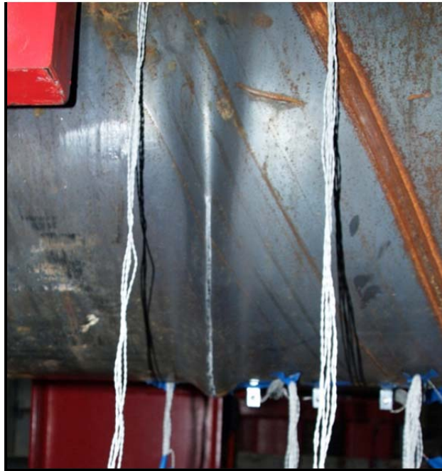
Figure 3-212: First rupture closed under compressive stress, en route ductility 6, \Delta=3.45 in
