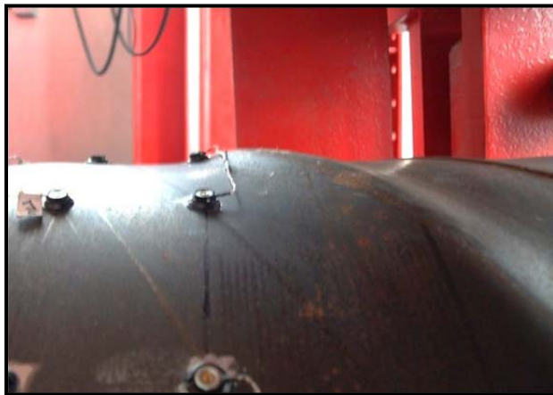
Figure 3-200: Buckle near loading point, ductility 3, \Delta=6.6 in
