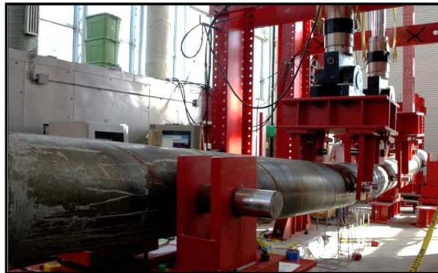
Figure 3-112: Pile profile, Ductility 4-1st push, \Delta=6.67 in.
