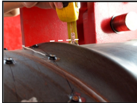
Figure 3-179: Buckle under loading point, ductility 4, \Delta = 8.0 inches
