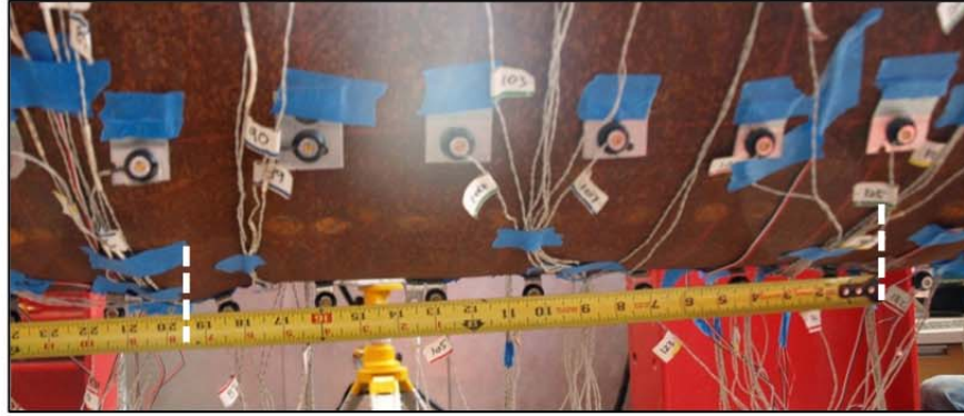
Figure 3-58: Spacing of buckles at ductility 3-pull 2, \Delta = 9.8 inches
