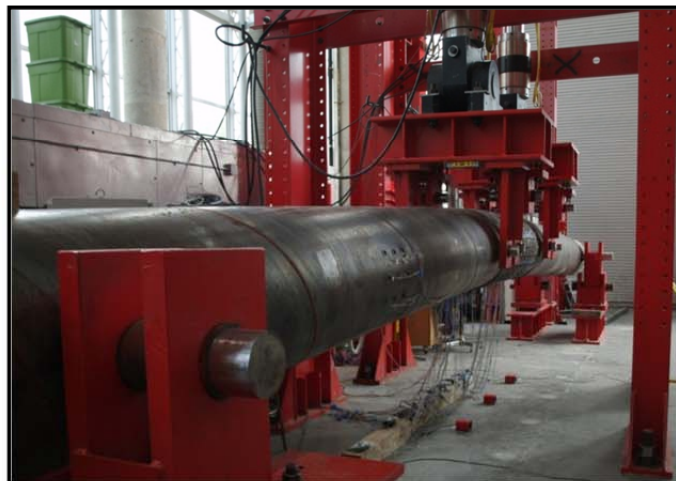
Figure 3-152: Pile with a mid-span displacement of 6.9 inches, ductility 3
