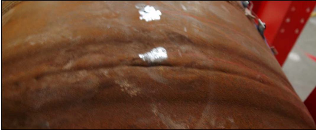
Figure 3-40: Necking of the pile, ductility six pull three, displacement = 12.8 inches
