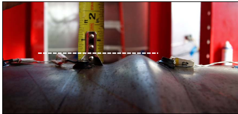
Figure 3-109: Buckle located in center of pile, Ductility 3-3rd push, \Delta=5.0\text{in}
