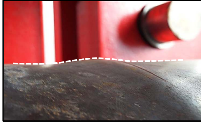
Figure 3-146: First buckling of the specimen, ductility 1.5, \Delta = 3.5 inches
