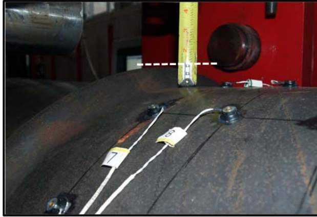
Figure 3-206: Buckle on the top of the pile under loading point, ductility 5, \Delta=11.1 in
