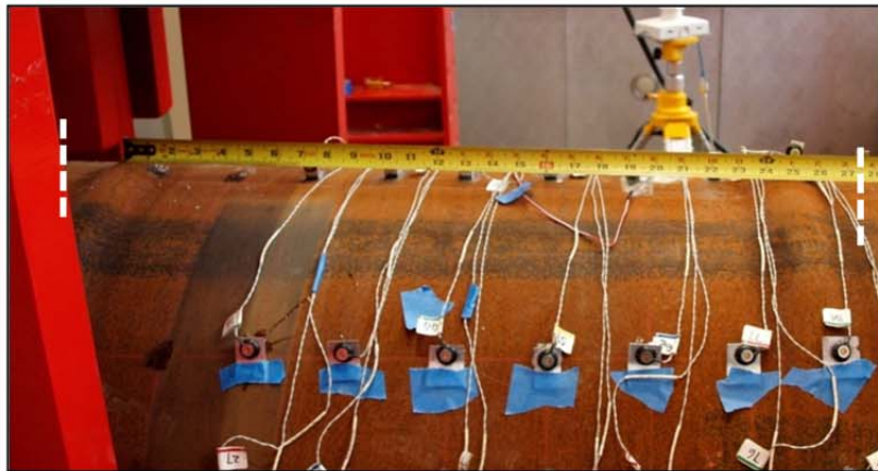
Figure 3-59: Spacing of buckles at ductility 3, \Delta = 9.8 inches
