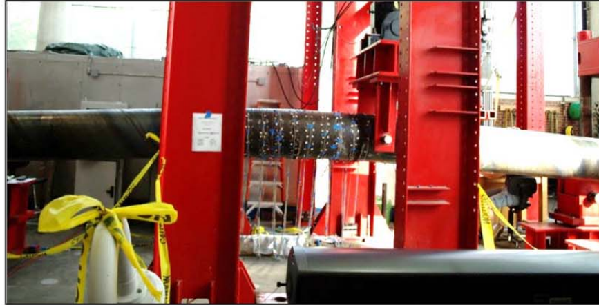
Figure 3-115: Pile Profile, Ductility 5-3rd pull, \Delta=8.33 in
