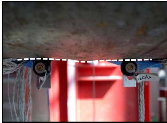
Figure 3-106: Pile buckle, Ductility 2-1st pull, \Delta=3.3 in
