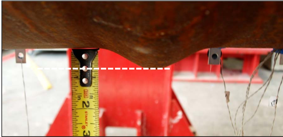
Figure 3-56: Buckle under loading point, ductility 3, \Delta = 9.8 inches
