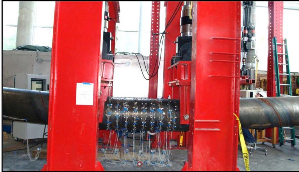
Figure 3-157: Pile with a mid-span displacement of 9.2 inches, ductility 4
