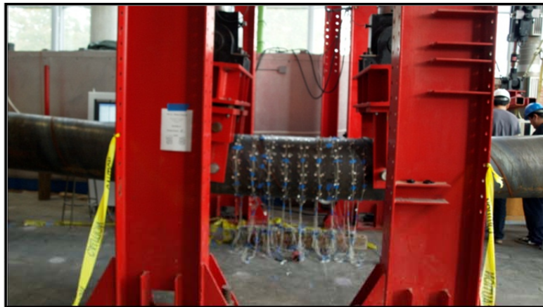
Figure 3-181: Specimen at maximum ductility displacement, ductility 5, \Delta = 10.0 inches
