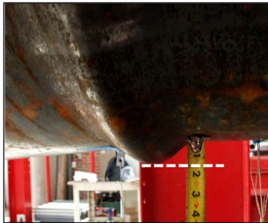
Figure 3-48: Buckle under the loading point during ductility four ( \Delta=12 inches)
