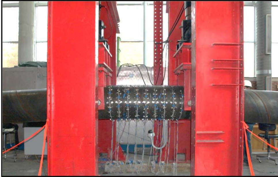
Figure 3-197: Deformed specimen, ductility 3, \Delta=6.6 in
