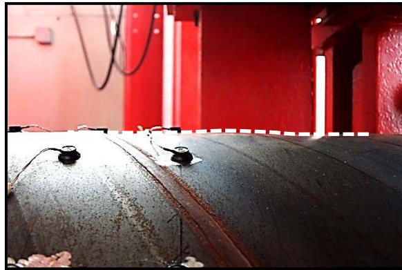
Figure 3-168: Initiation of buckling, ductility 2, \Delta = 4.0 inches
