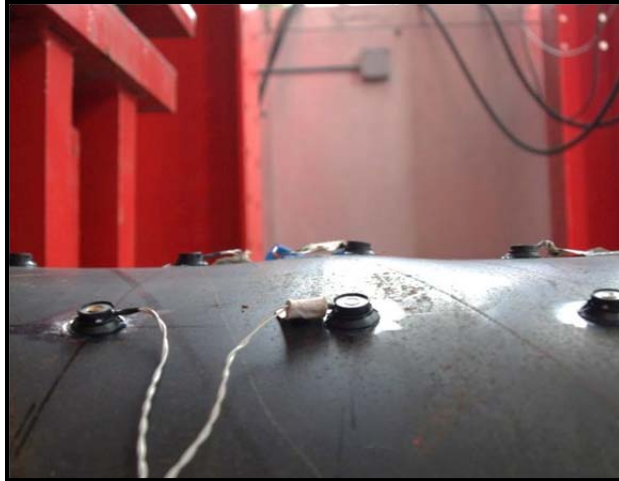
Figure 3-199: Buckle in constant moment region, ductility 3, \Delta=6.6 in
