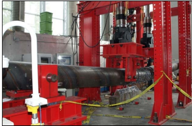
Figure 3-94: Pile profile, Ductility 5, \Delta = 9.4 in
