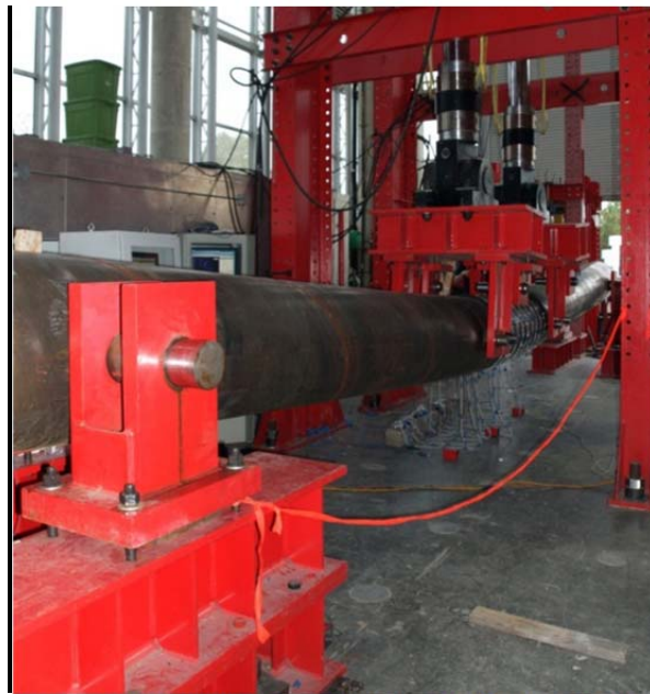
Figure 3-205: Deformed specimen, ductility 5, \Delta=11.1 in
