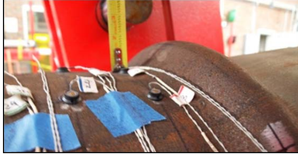
Figure 3-75: Buckle under North loading point during ductility seven, \Delta = 18.2 in
