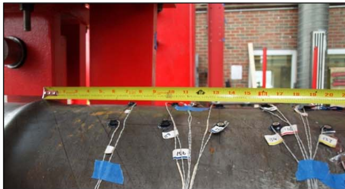
Figure 3-92: Buckles spaced evenly (17-20" apart), Ductility 3, \Delta = 5.6 in
