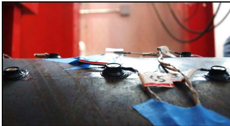
Figure 3-127: Formation of buckle 12 in. north of centerline; ductility 1.5 push 2, \Delta=4.2 in
