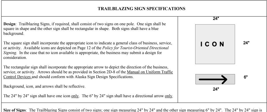
**Size of Signs**: The Trailblazing Signs consist of two signs; one sign measuring 24" by 24" and the other sign measuring 6" by 24". The 24" by 24" sign is located above the 6" by 24" sign on the same pole. Vertical spacing between the two signs shall be two inches. The sign panel thickness shall be 0.125 inches. All posts shall be 2 1/2 inch perforated steel tubes. All posts shall be installed in sleeve type concrete foundation.
