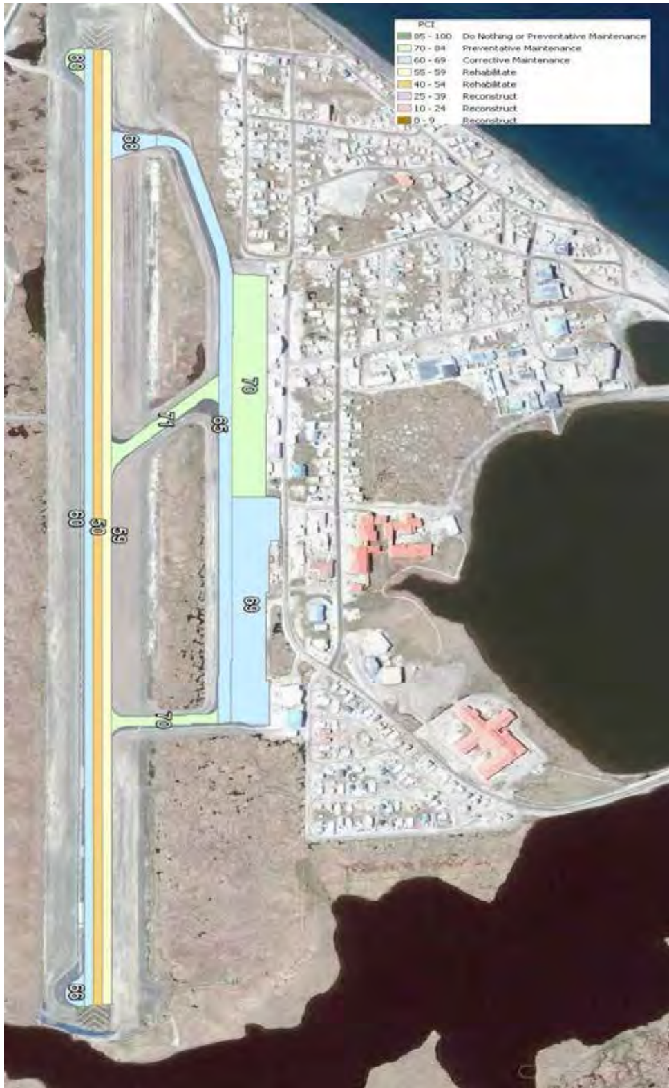
Barrow Airport Pavement Condition Index Map
