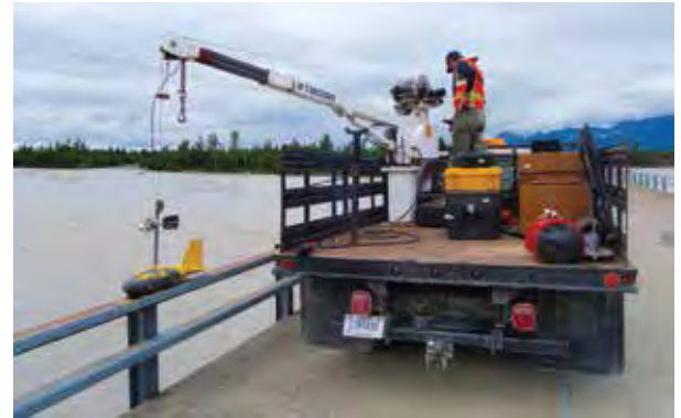
Placing a 300 lb. depth and current monitor in the Copper River. Photo by Mike Knapp, ADOT&PF.
