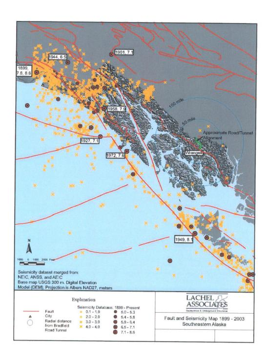
Figure 3-2: Regional Seismicity
