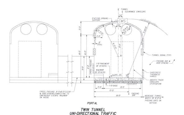
Figure 4-1: Layout of Twin Uni-Directional Tunnel
