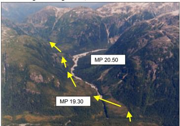
This segment of conceptual alignment contains many challenges for the construction of a transportation corridor. Due to the steep valley slopes, hard granitic rock, and five locations that require bridges, the excavation process will be costly and time consuming. More refined engineering may be able to reduce the excavation quantities but there are limited areas where excess excavation can be used, and some long hauls may be necessary.
