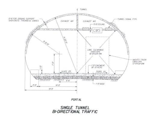
Figure 4-2: Layout of Single Bi-Directional Tunnel
