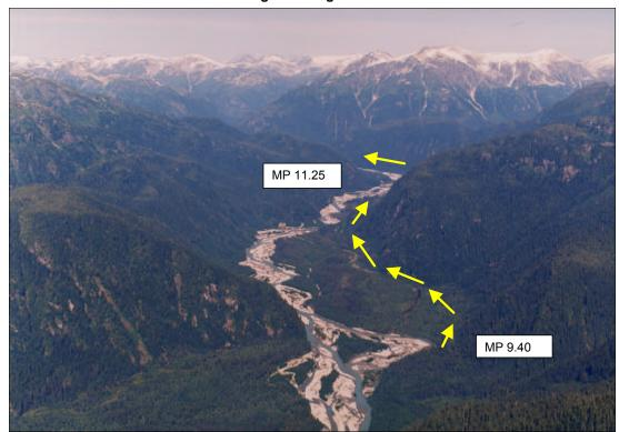
The abandoned logging road is still visible in many areas, meandering thru the floodplain. This segment of proposed new alignment is conceptualized in a more stable location, and is anticipated to require approximately 1.4 million cubic yards of excavation. Further evaluation and engineering should reveal opportunities to reduce the excavation quantities, but the steep side slopes along this segment will keep the costs of road construction high.
