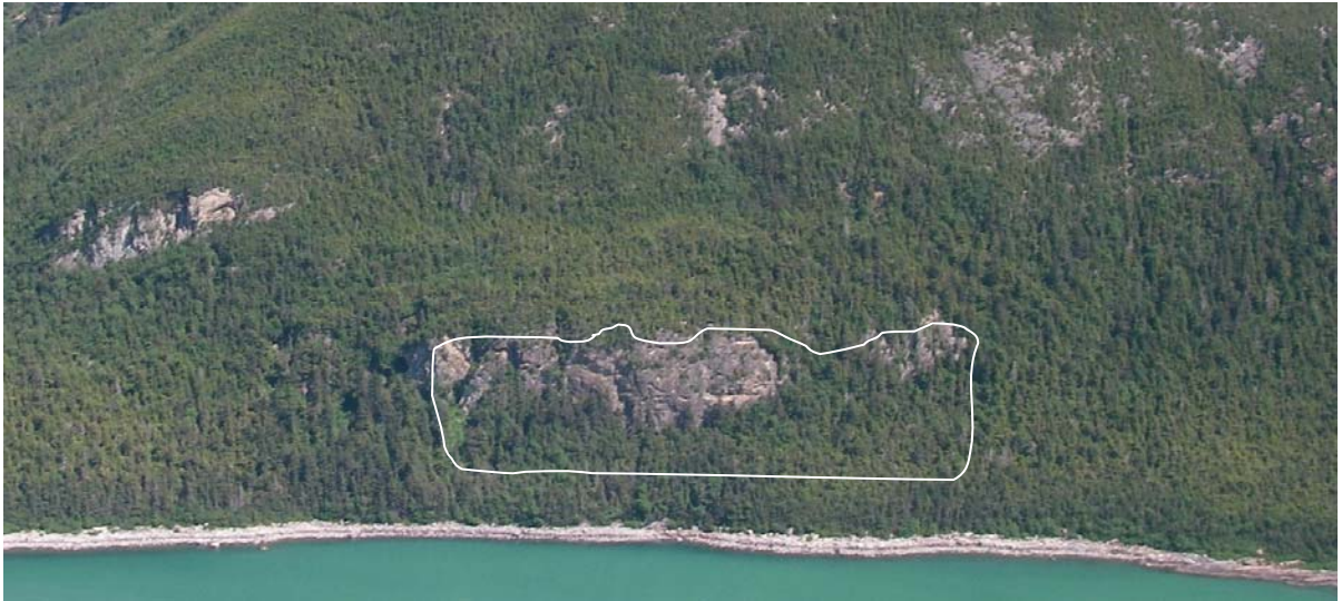
RF14. View east/upslope at moderate rockfall hazard from IRP 2006 1933+00 to 1953+00, below massive gneiss cliffs.
