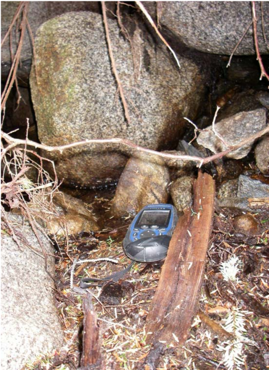
Colluvium (Qc) - View of typical colluvial material. Material is angular to subrounded and multi-lithic. Handheld MobileMapper™ is 3 inches wide for scale. Photo taken 75 ft right of IRP 2006 2008+50.
