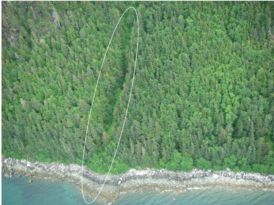
DF03. View east/upslope at debris flow channel, deposition zone, and fan near IRP 2006 1518+00.
