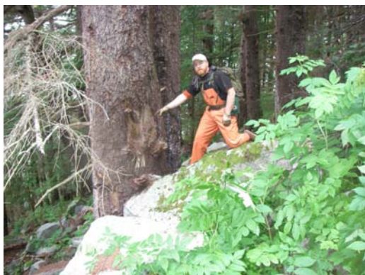
RF32. View north/up alignment at scar on tree from rockfall/boulder striking tree. Photo taken at centerline at IRP 2006 2364+50.
