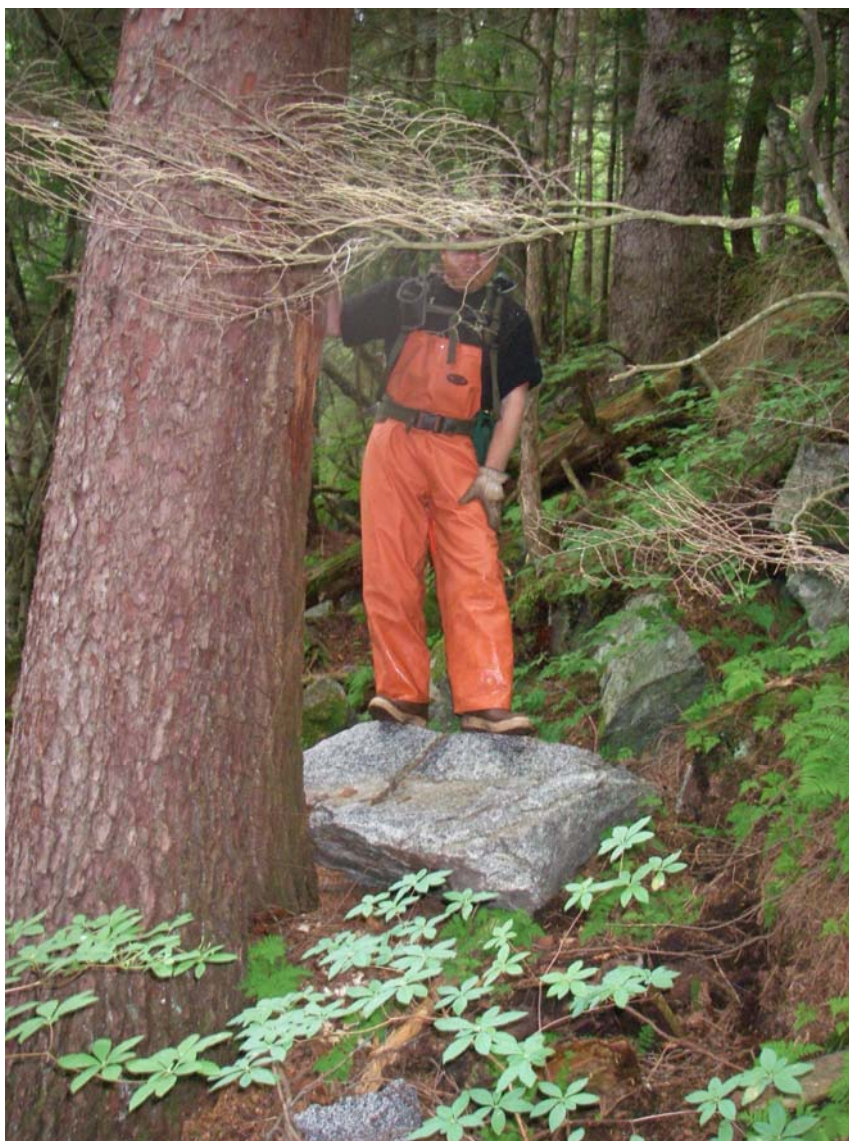
RF33. View north/up alignment at a 300-500 lb boulder/rockfall (fresh) from cliffs above, stopped by a tree. Photo taken at centerline at IRP 2006 2367+00.
