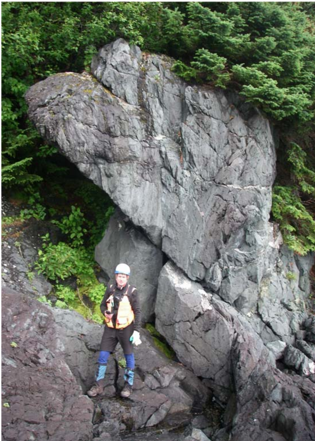
Basalt bedrock (Bxv) - view of typical basalt bedrock outcrop. Note massive appearance and multiple joint sets. Photo taken 15 ft left of IRP 2006 1716+00.
