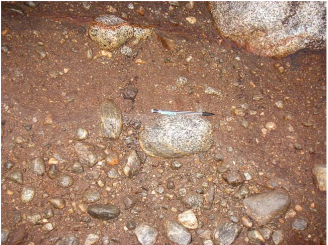
Glacial outwash deposits (Qgo) - View of typical glacial outwash deposit. Pencil approximately 6 inches long for scale. Photo taken 120 ft right of IRP 2006 2427+00.
