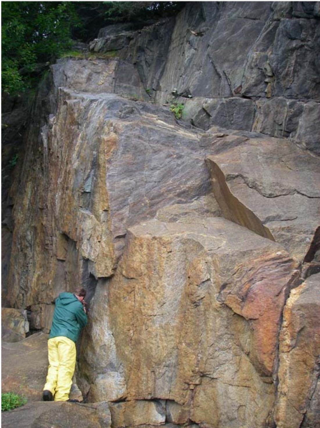
Undifferentiated metamorphic bedrock (Bxm) – View east at a shoreline cliffs greater than 40 ft high, with banded gneiss and metasedimentary bedrock (quartzite and metamorphosed carbonate observed.) Photo taken on centerline at IRP 2006 2106+75.
