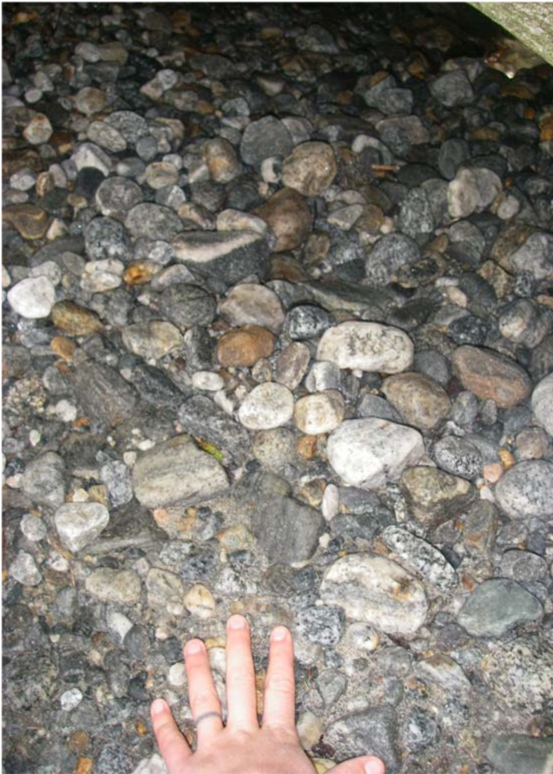
Elevated beach deposits (Qeb) - View of typical elevated beach deposit material. Photo taken 490 ft right of IRP 2006 2418+00.
