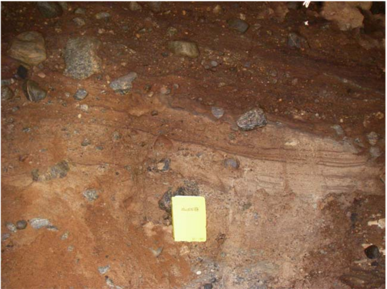
Glacial outwash deposits (Qgo) - View of typical glacial outwash deposit. Note stratification of sands. Field book approximately 5.5 inches wide for scale. Photo taken 120 ft right of IRP 2006 2427+00.
