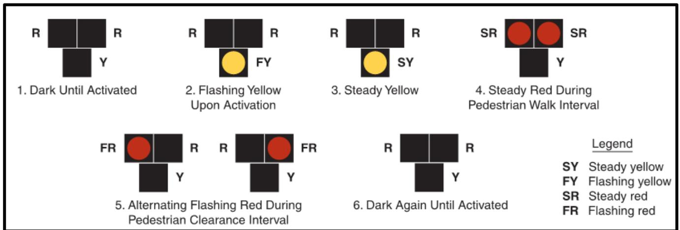
Figure 3 The PHB Operation Sequence (From MUTCD Figure 4F-3)
