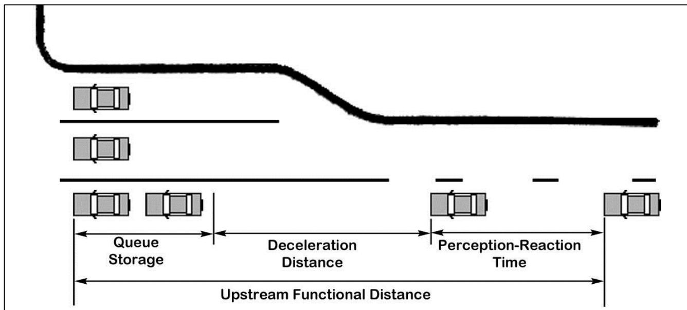
Figure 2 – Components of Upstream Functional Distance
