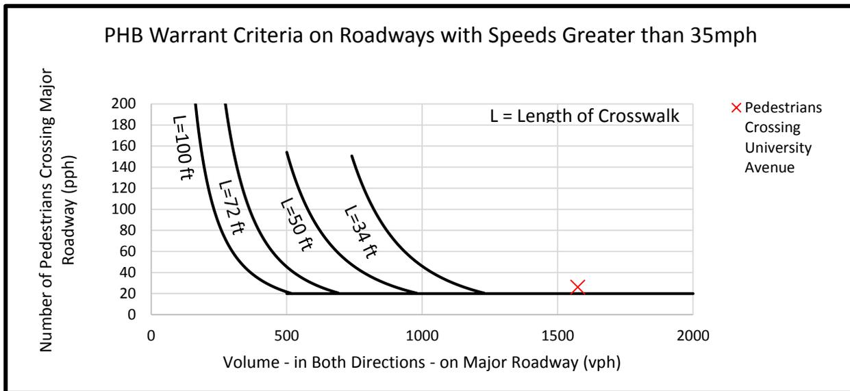
**Figure 4 Warrant Criteria for Installing a Pedestrian Hybrid Beacon (Adopted from the MUTCD Figure 4F-2)**
