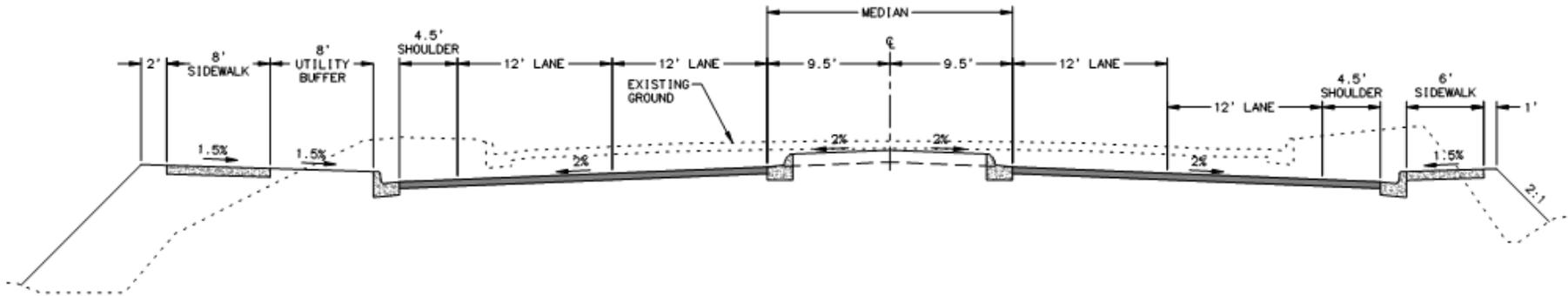
Figure 12: University Avenue Proposed Design Typical Section
