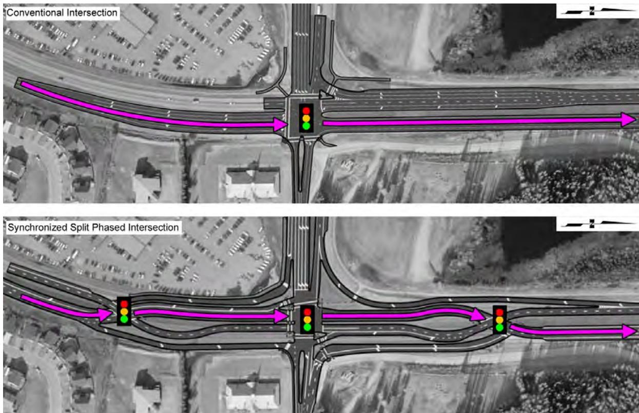
**Figure 12: Northbound Vehicle Movement, Conventional Intersection Versus Synchronized Split-Phased Intersection**
