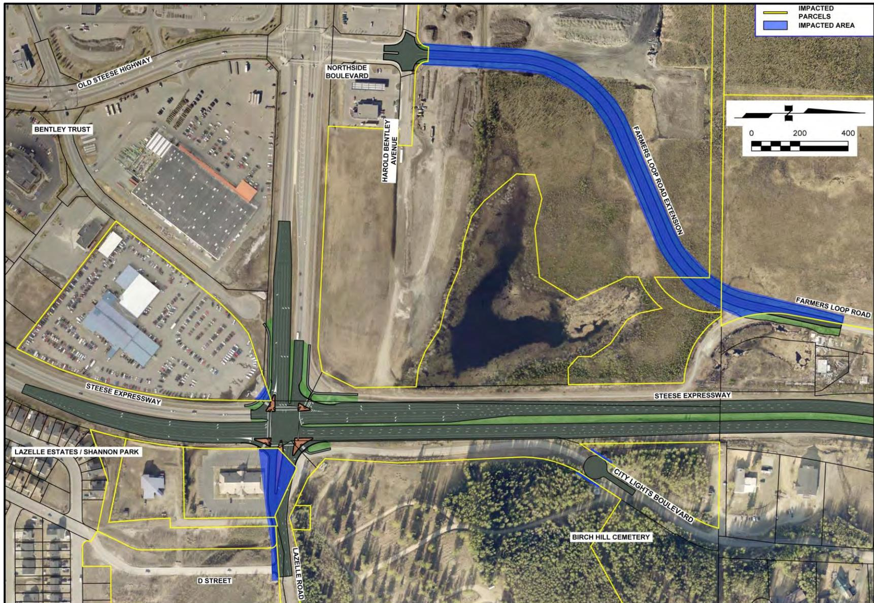
Figure 51: ROW Impacts for Alternative E, Old Steese to Farmers Loop Connection with Relocation of Fort Wainwright Gate
