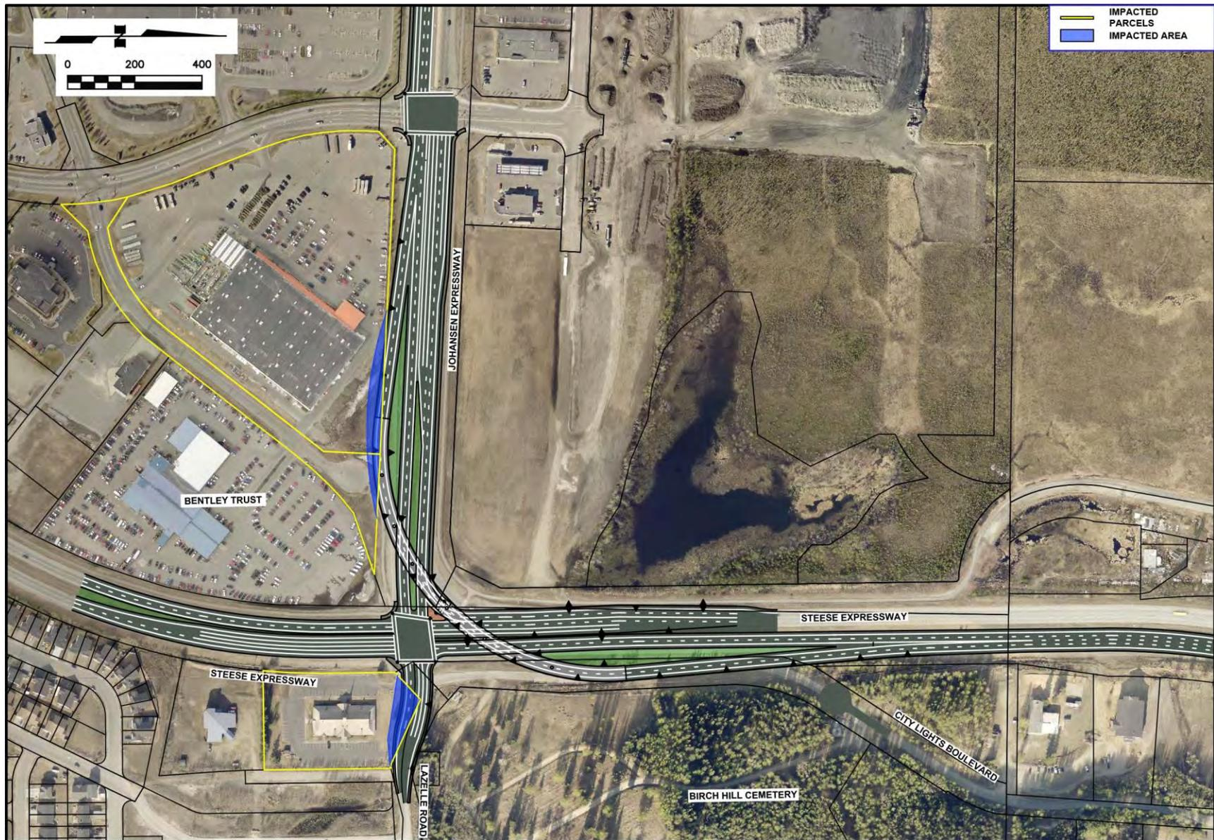
**Figure 59: ROW Impacts for Alternative F, Eastbound Left Turn Flyover with Relocation of Fort Wainwright Gate**
