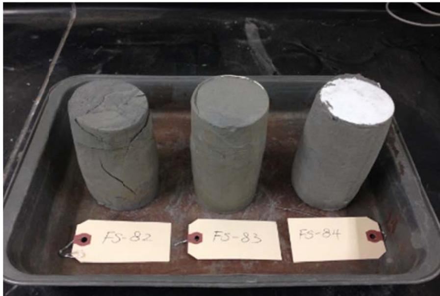
**Figure 2.15 Samples after Isotropically Consolidated Undrained Test**
