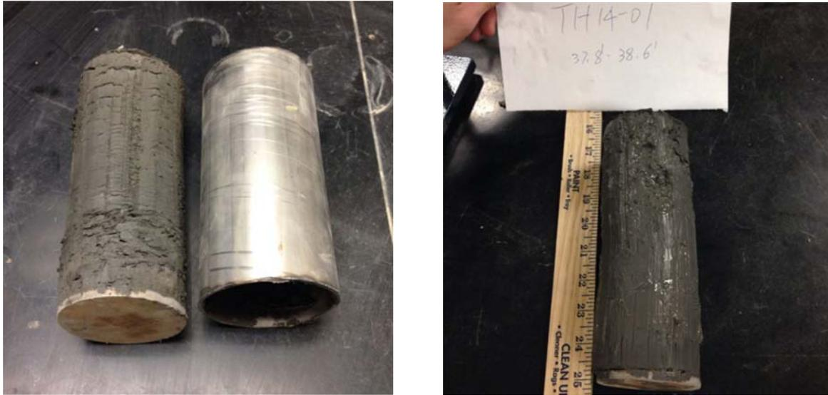
**Figure 2.1 Soil Sample Extraction with Cutting Disc**
