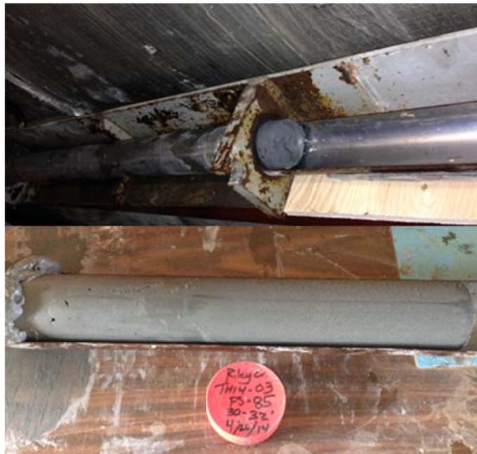
**Figure 2.2 Soil Sample Extraction with Hydraulic Extruder**
